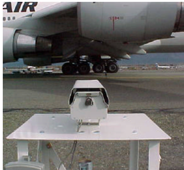
Laser measuring the distance of the nose gear from the centerline.
