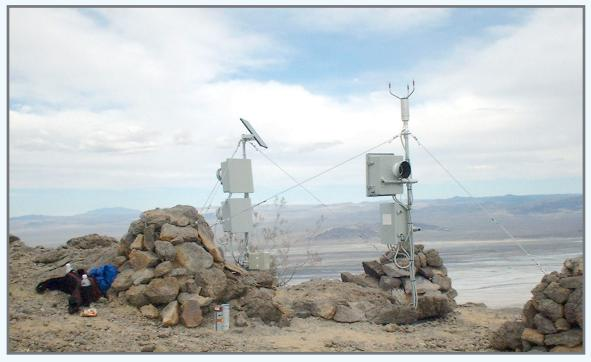
Automated Remote Digital Imaging System (ARDIS) is a means of automatically acquiring color digital images of dust storms. The images are used to determine the directions from which dust particles become airborne, t intensity and duration of the dust event, and the meterological conditions at time, in conjunction with nearby CLIM-MET stations. The system is placed of top of a mountain to provide views of dust events from 9-20 km away.
