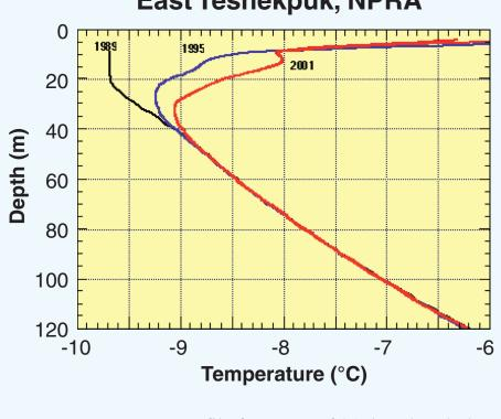
Temperature profile from one of 21 deep boreholes in the NPRA array showing the response of permafrost to the significant warming of the 1990's.
