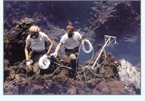
USGS researchers collecting samples from the Pu'u O'o vent of the Kilauea Volcano, Hawaii, to determine the kinds and amounts of gases and particles emitted.
