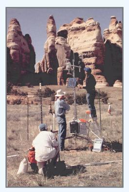
IM-MET stations are terological/geological stations that a signed to function in remote areas for ng periods of time without human tervention. These stations monitor weath variables including temperature, wind, and precipitation; site variables including soil noisture and temperature, and eolian ticle movement; and collect samples of analyses. Data are automatically recorded at regular intervals.
