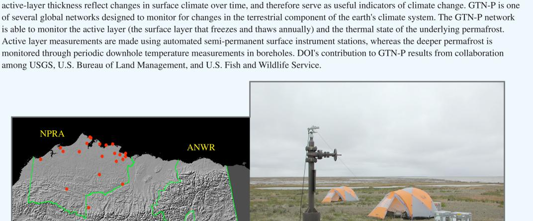
The subsurface permafrost monitoring network currently covers federal lands in and near the National Petroleum Reserve Alaska (NPRA Subsurface temperatures are measured periodically with downhole sensors that indicate the depth and thickness of the active layer and permafrost, and yield subsurface temperature profiles. These measurements are important for determining the long-term terrestrial response
