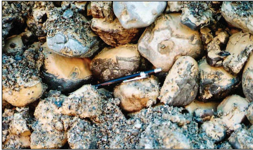
Figure 81. —Naturally occurring segregated soil. During deposition, the gravel sizes were segregated from the sand sizes. Poor construction practices can lead to similar segregation. The deposit is a broadly graded mixture of silt, sand, and gravel and is internally unstable. Note that silt has eroded into the gravel sizes and coated the particles.
