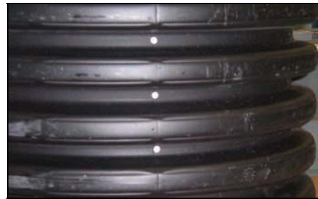
Figure 55. —Profile wall corrugated HDPE pipe with circular perforations.
