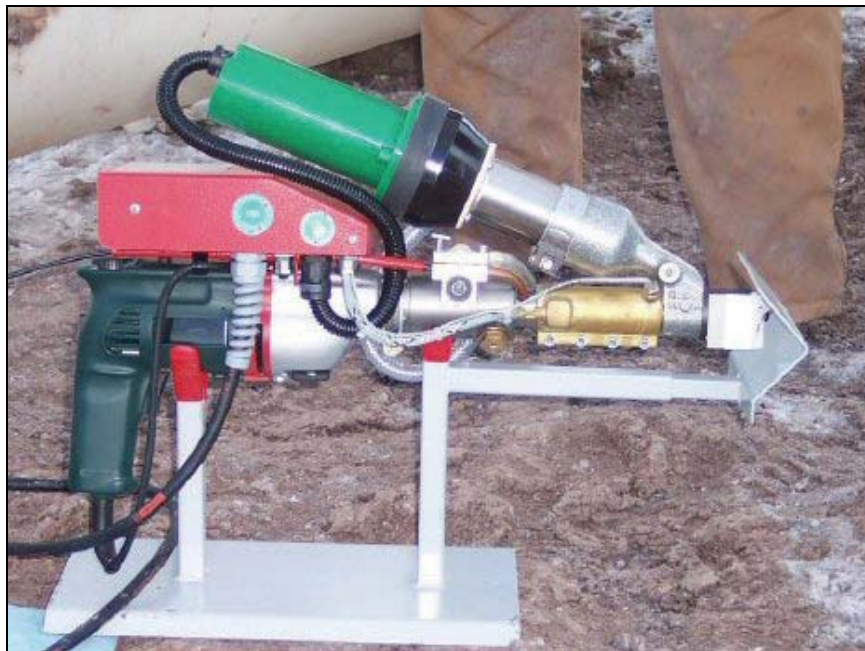
Figure 11.—Hand held extrusion gun.
