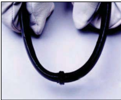
Figure 10. —A butt fused HDPE pipe joint being checked for gaps and voids.
