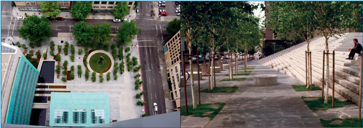
Figure 5-23: Use of planting to soften and enhance the appearance of walls and other security elements at the Seattle Courthouse.
