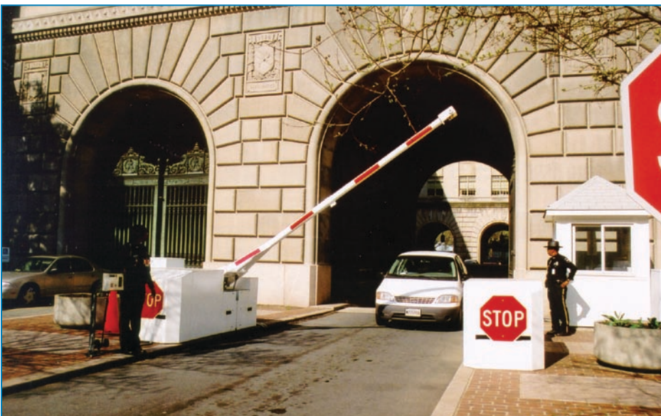
Figure 4-42: Drop-arm crash beam.
