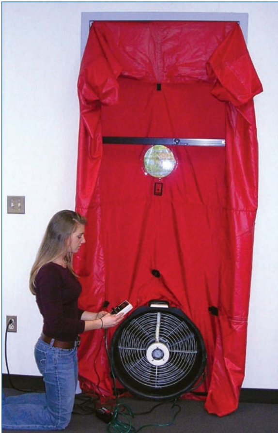
Figure 3-5 A blower door test on the selected safe room aids in estimating the size of air-filtration unit required and in identifying air leakage paths.
