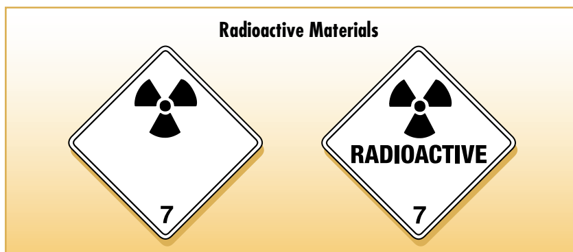
Figure 5-16 Placards associated with radiological incidents
