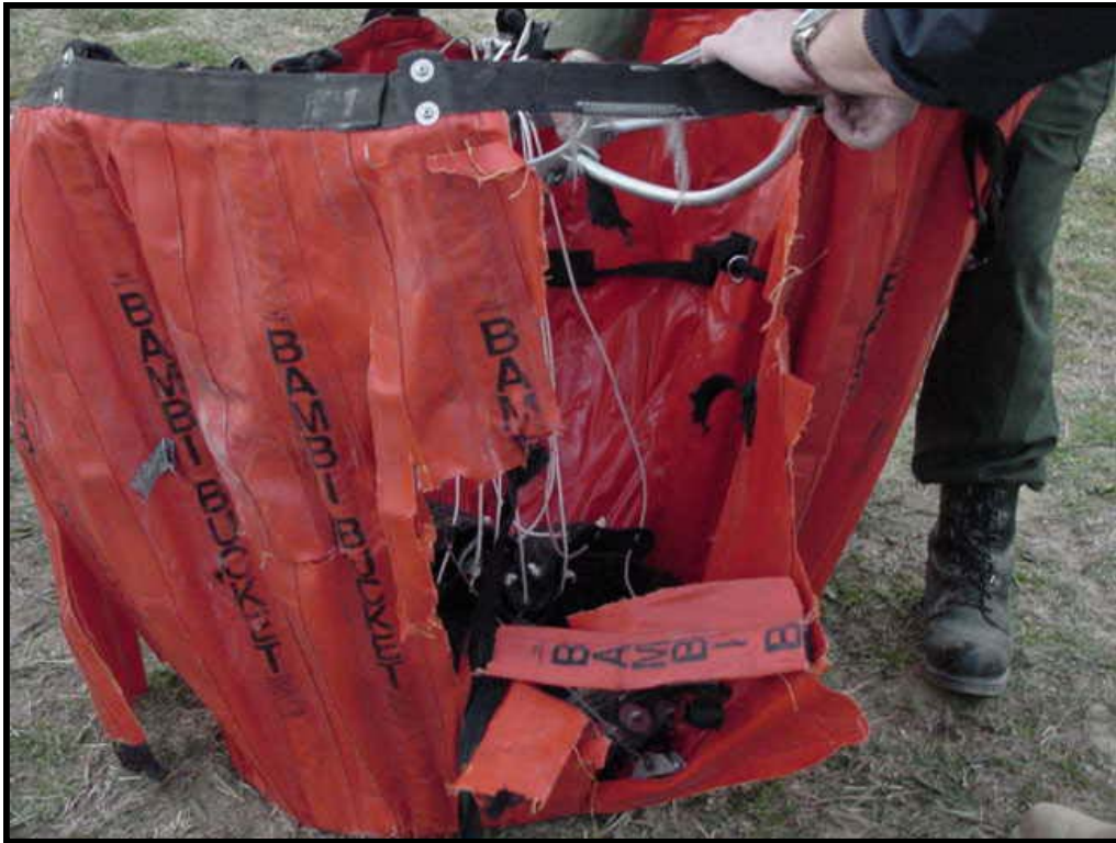
The total length of cable and bucket was 25 feet. The distance from the cargo hook to the tail rotor blade was 20 feet 2 inches.
