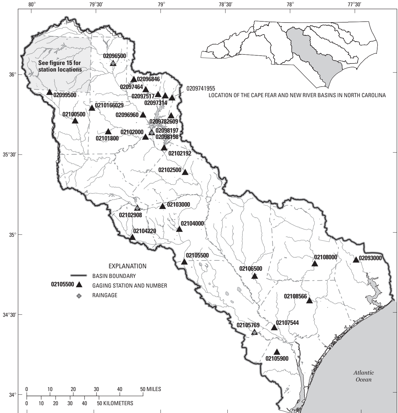
Figure 6. Locations of surface-water stations in the Cape Fear and New River Basins, North Carolina.
