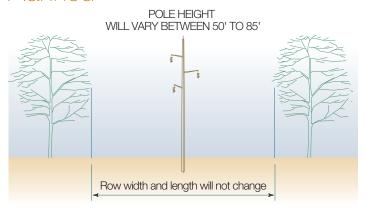
The new structures will be of wood-laminate construction. Their height will average about 50 to 85 feet above ground, slightly below surrounding tree height. The existing right-of-way will not be changed, however, because the corridor will be trimmed and cleared as necessary in order to meet electrical clearances for safety and reliability, in many locations it will appear to be wider.
