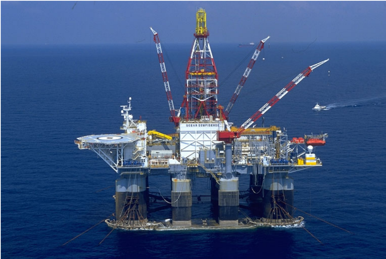
Figure 27a. – The Ocean Confidence , a Class III, dynamically positioned, submersible drilling rig. However, anchors may be deployed for some applications. (Photograph courtesy of Diamond Offshore Drilling, Inc.)
