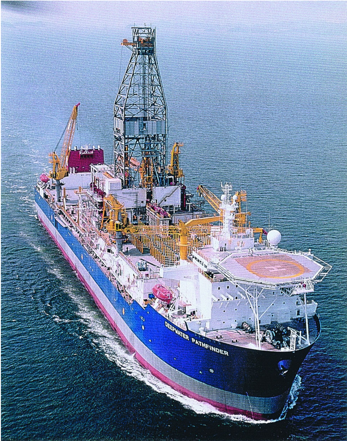
Figure 27b. – The Deepwater Pathfinder , a dynamically positioned drillship (Photograph courtesy of Transocean SedcoForex).
