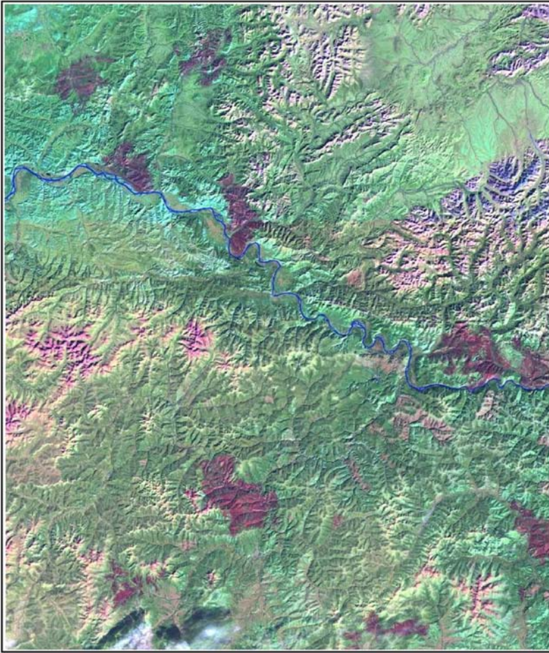
Figure LA-3 —This mosaic of two Landsat 7 ETM+ scenes from 12 Sept 1999, shows the Yukon Charlie region of Alaska. Nine large burns are clearly visible (dark purple) from fires earlier in the summer. This type of remote sensing data allows managers to discover details of burns, which because of daunting logistics, may never be visited on the ground. The challenge has been to find the best measure of severity from such data, and to develop protocols that offer standardization, so burns can be compared spatially and temporally.
