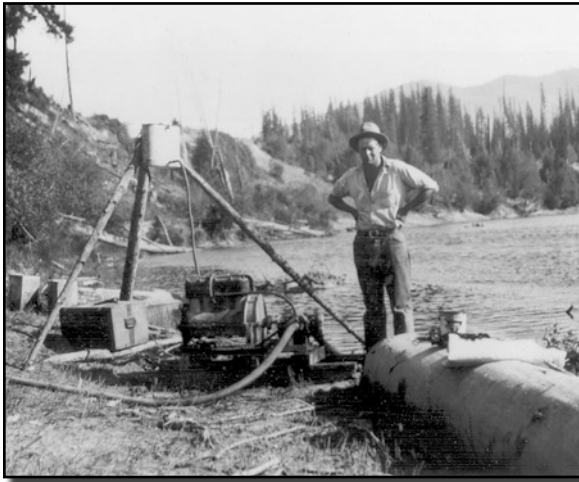
A "Pacific Pump" was used in 1938 at Benton Creek to provide water to control an experimental broadcast burn in studies of slash disposal. The Benton Creek drainage later was instrumented to make it a model watershed. (Gisborne collection, 98(vii): 662)
