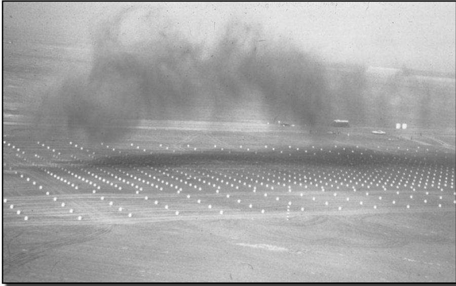
Hundreds of cups collected fire retardant from test drops to provide data on coverage patterns and concentrations of the liquid in various parts of the drop area.
