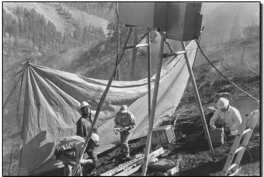
Station research engineers collected sediment washed off a burned hillside plot by an artificial rain simulator in 1995 as part of a study in the Boise River drainage.
