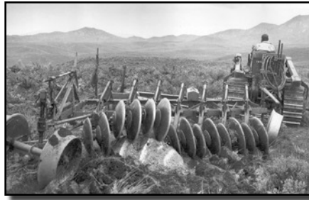
Station and DWR researchers led by Perry Plummer evaluated equipment such as the "Australian stump-jump plow" for preparing seedbeds on depleted rangelands. The plow's disks could jump up to allow rocks and debris to pass underneath.
