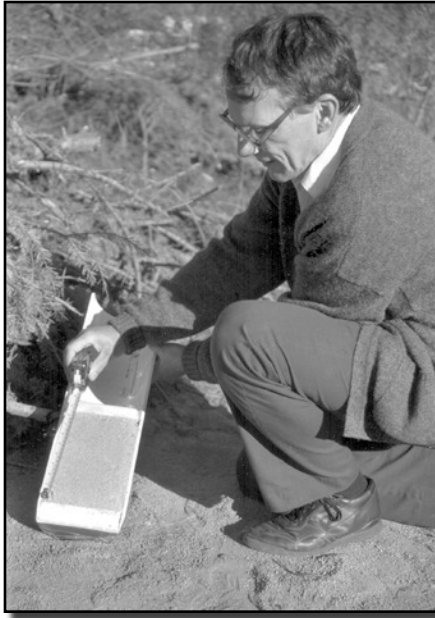
Project Leader Ed Burroughs searched for a fire-induced hydrophobic soil layer in 1991 in one of the many types of research the engineering technology unit conducted.
