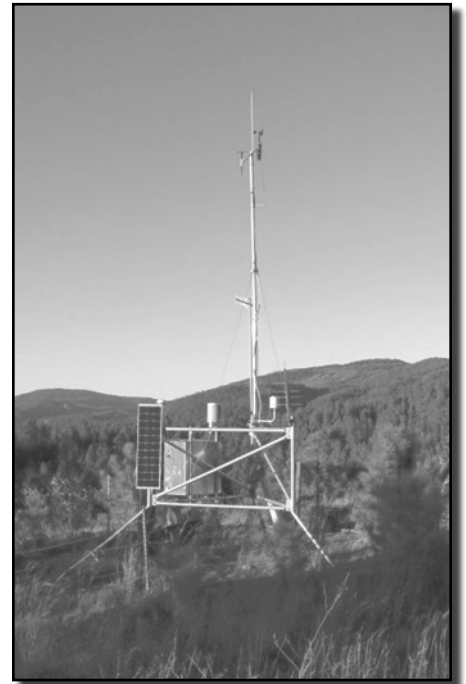
Station researchers did early work in developing Remote Area Weather Stations that could feed climate data from remote locations via satellite to fire planning and management personnel.
