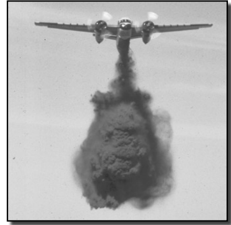
Fire Lab researchers studied the efficiency of various aircraft and the effects of different types of retardants and delivery systems in retardant drop tests, such as this one in 1983.
