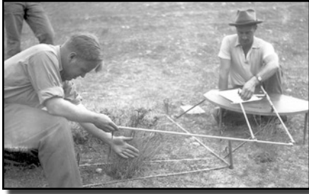
Ken Pearse (left) and an unidentified assistant demonstrated the improved pantograph he and Joe Pechanec developed.
