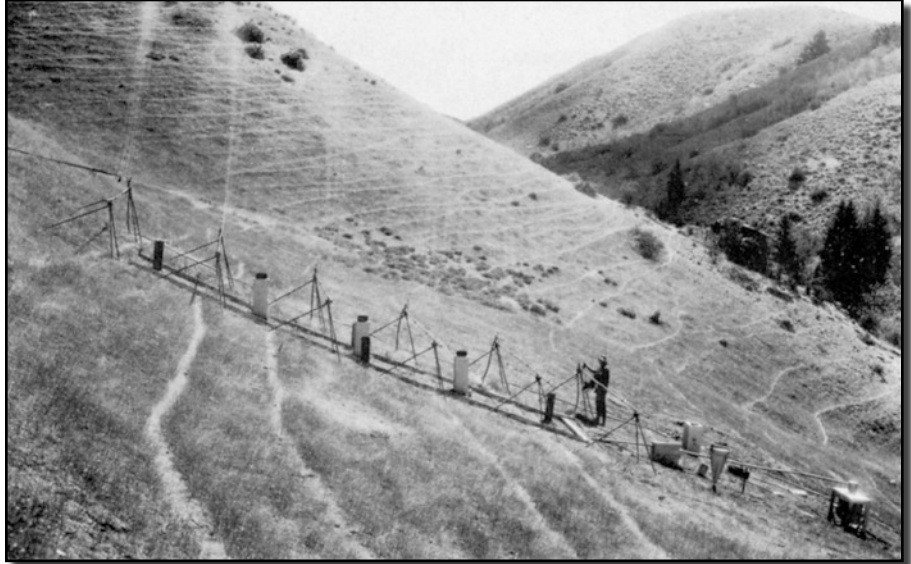
Artificial rainmaking equipment designed by Ken Pearse was set up to measure surface erosion from this Idaho rangeland that had been heavily overgrazed by domestic sheep.
