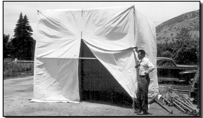
Station Watershed Scientist Paul Packer provided information that helped the Forest Service prevail in controversies over reducing grazing in the Idaho Batholith. Here, Packer checked infiltrometer equipment used to simulate rainfall in hydrologic studies at Wood Tick Creek in the Boise National Forest in 1947.
