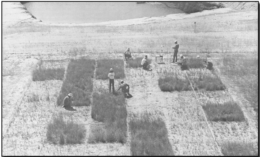
Station researchers planted various seed mixtures and used different fertilizer, irrigation, and mulch treatments on study plots located on graded spoils at the Decker Coal Mine in southeastern Montana.
