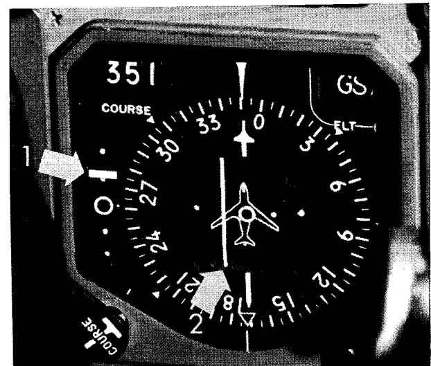
FIGURE 5. The Collins 331A-7 course deviation indicator (CDI) provides glide slope, localizer, and heading information. According to the positions of the glide slope needle (arrow #1) and the localizer needle (arrow #2), the aircraft is below glide slope and to the right of the localizer by one dot.
