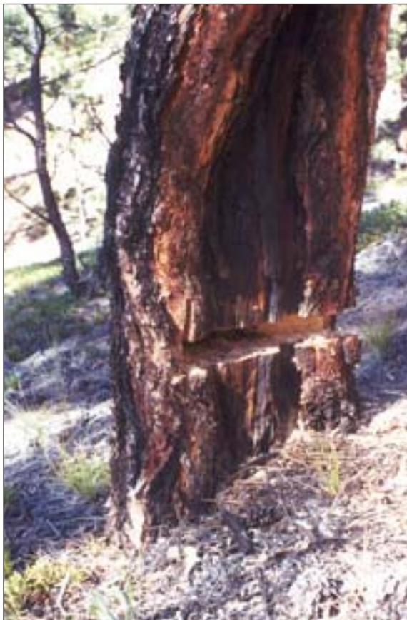
6b. Fire scars can be sampled from living trees by cutting out a partial section through the scar face.
