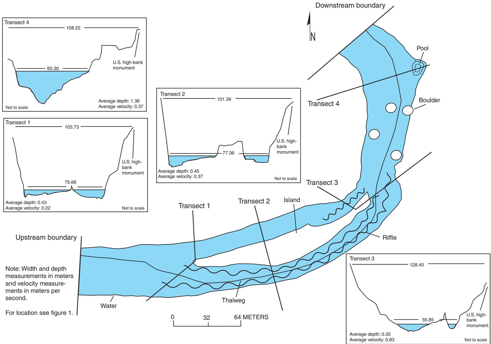
Figure 5. Planimetric reach map for Rio Grande above Boquillas Canyon.
