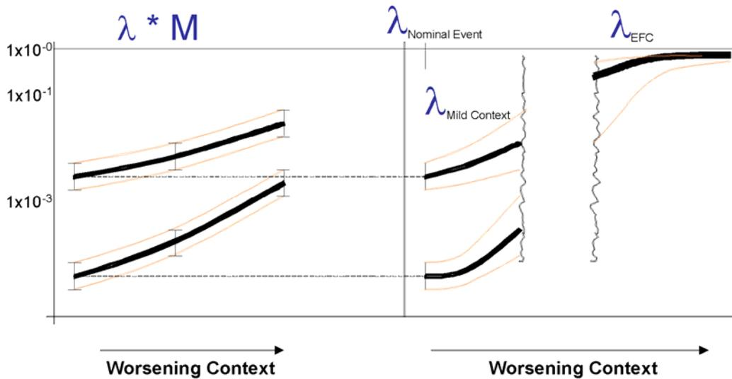
Figure 18 Possible Models for Human “Error” Rate Variability.
