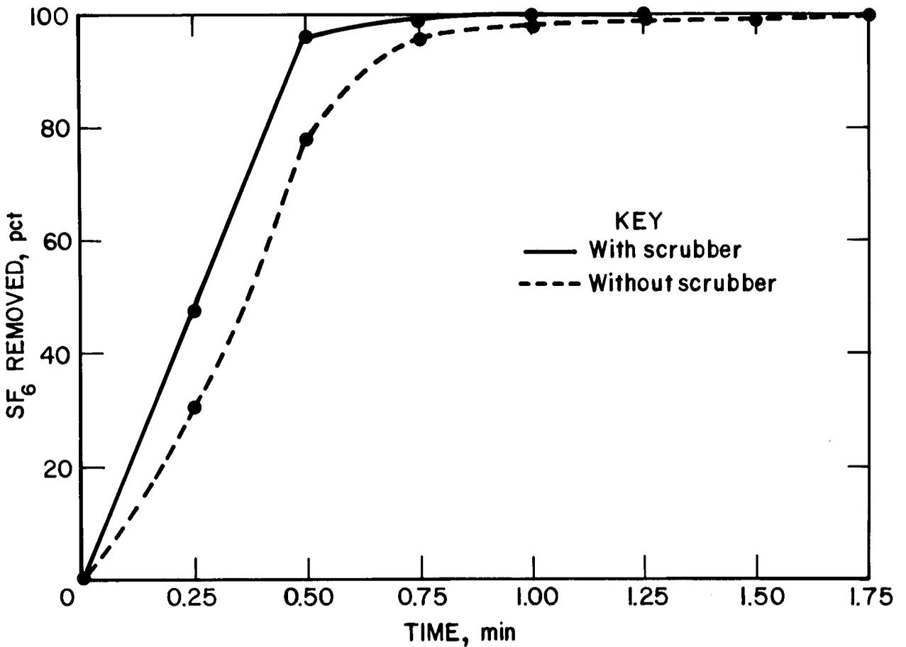
FIGURE 16. - SF<sub>6</sub> scrubber comparison at 6,000 cfm with 10-ft curtain setback.
