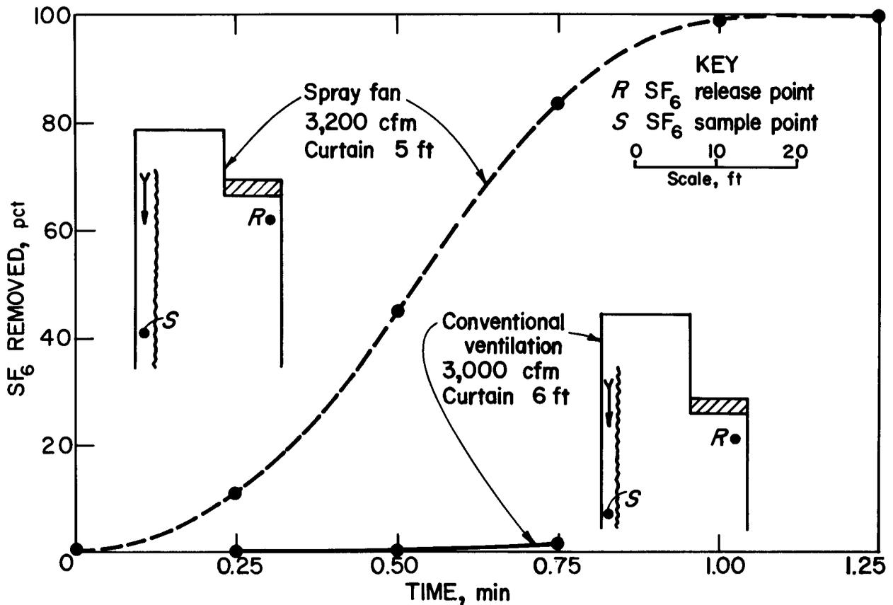
FIGURE 10. - SF<sub>6</sub> spray fan comparison in a slab cut configuration
