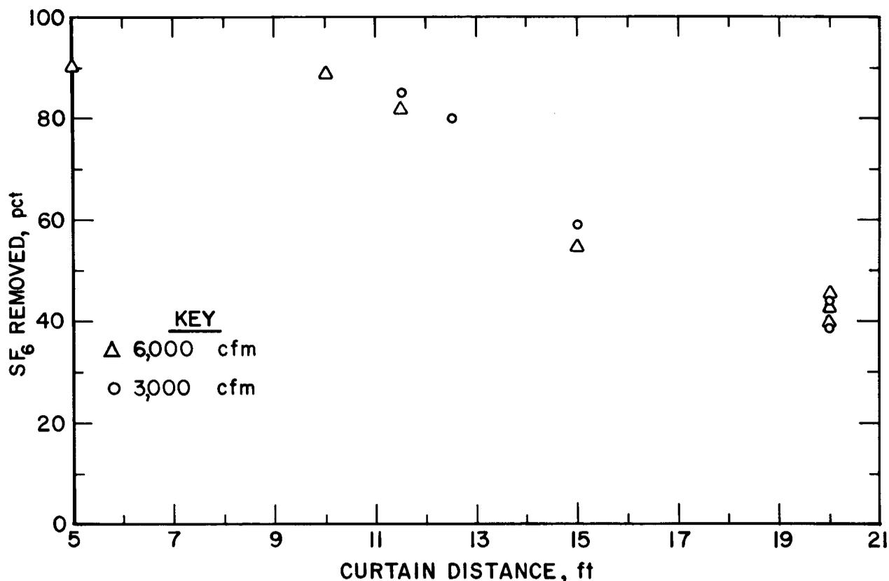
FIGURE 5. - Percent  $SF_6$  removed in 1 min with respect to curtain distance.
