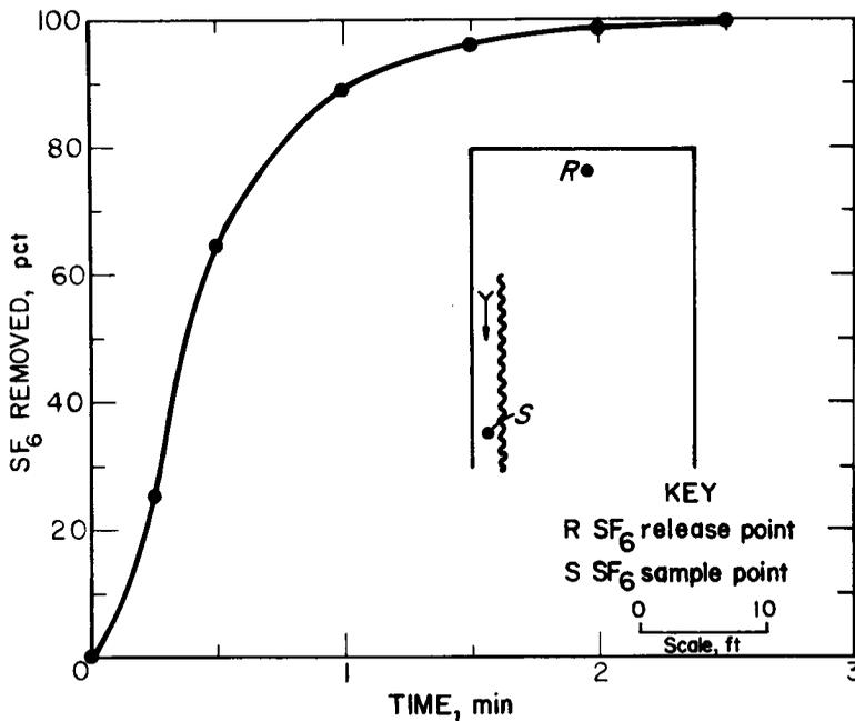
FIGURE 2. - Percent SF<sub>6</sub> removed at 6,000 cfm with 10-ft curtain setback.
