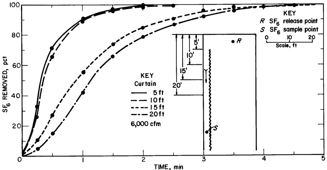
FIGURE 4. - Percent SF<sub>6</sub> removed at different curtain distances.
