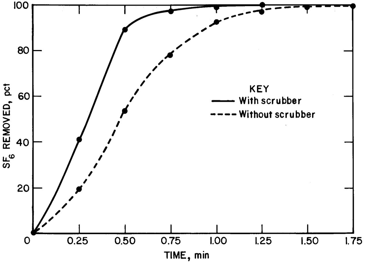
FIGURE 18. - SF<sub>6</sub> scrubber comparison at 6,000 cfm with 20-ft curtain setback.
