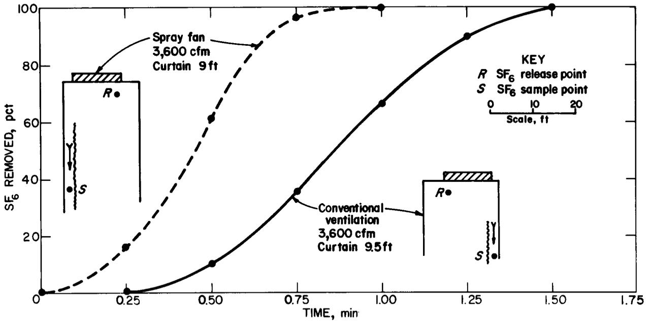
FIGURE 8. - SF<sub>6</sub> spray fan comparison at beginning of a box cut.
