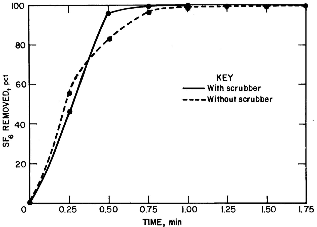
FIGURE 21. - SF<sub>6</sub> scrubber comparison at 9,000 cfm with 20-ft curtain setback.
