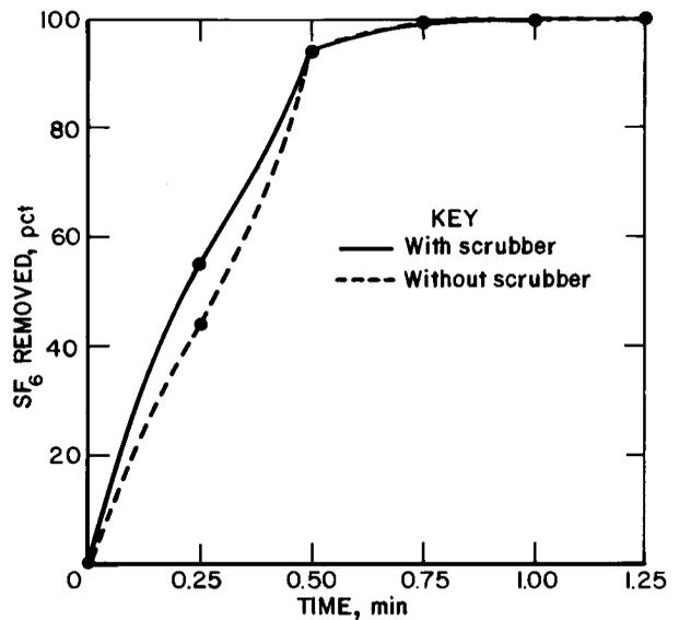
FIGURE 20. - SF<sub>6</sub> scrubber comparison at 9,000 cfm with 15-ft curtain setback.
