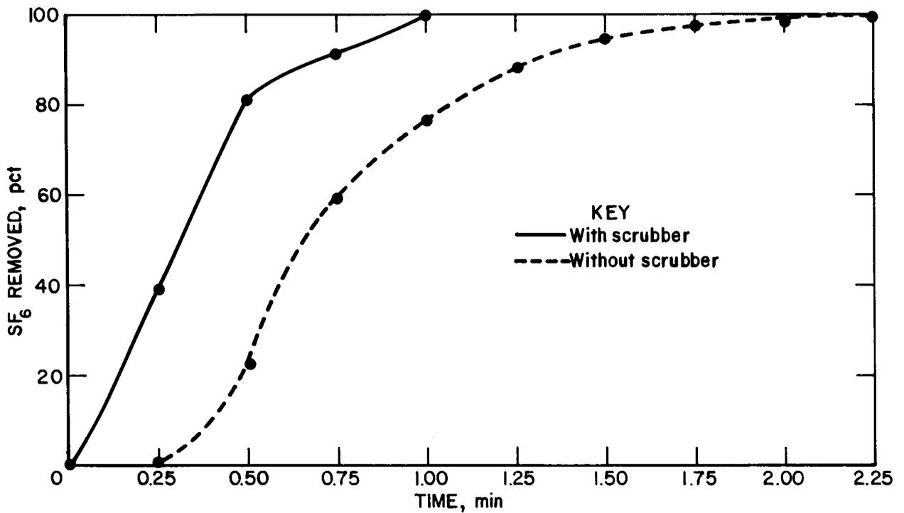
FIGURE 14. - SF<sub>6</sub> scrubber comparison at 3,000 cfm with 20-ft curtain setback.
