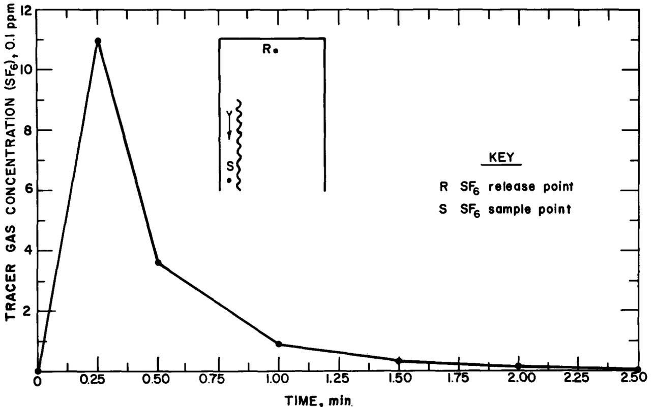
FIGURE 1. -  $SF_6$  concentration with respect to time (6,000 cfm, 10-ft curtain setback).
