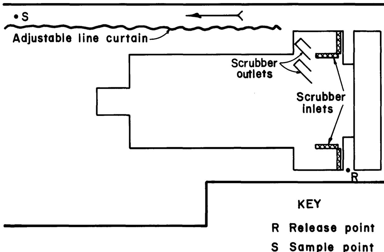
FIGURE 12. - Test configuration for evaluating dual-scrubber system.
