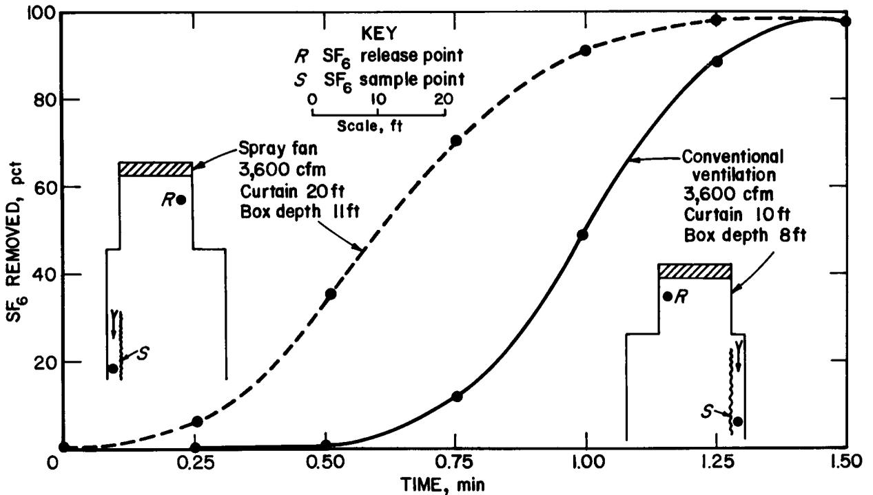
FIGURE 9. - SF<sub>6</sub> comparison of the spray fan with 20-ft curtain setback and conventional ventilation with 10-ft curtain setback.
