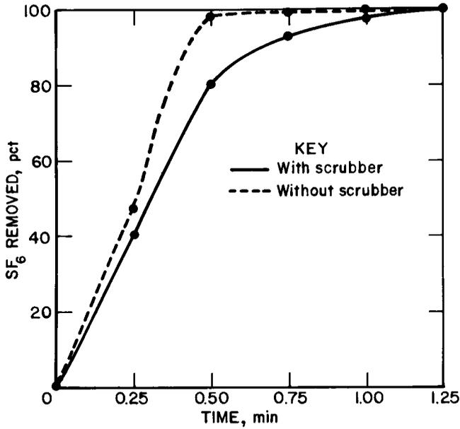
FIGURE 15. - SF<sub>6</sub> scrubber comparison at 6,000 cfm with 5-ft curtain setback.
