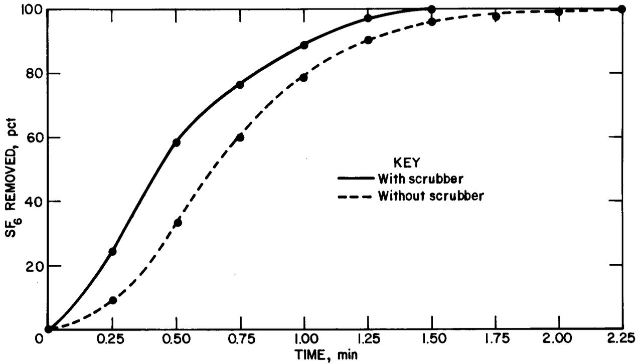
FIGURE 13. - SF<sub>6</sub> scrubber comparison at 3,000 cfm with 15-ft curtain setback.
