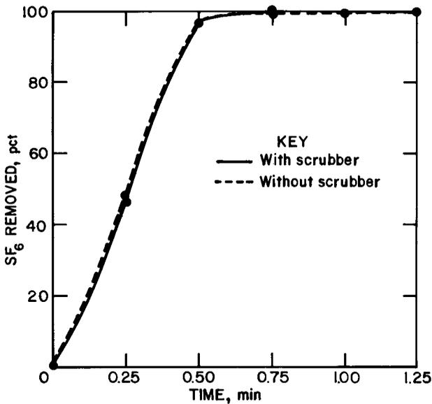
FIGURE 19. - SF<sub>6</sub> scrubber comparison at 9,000 cfm with 10-ft curtain setback.
