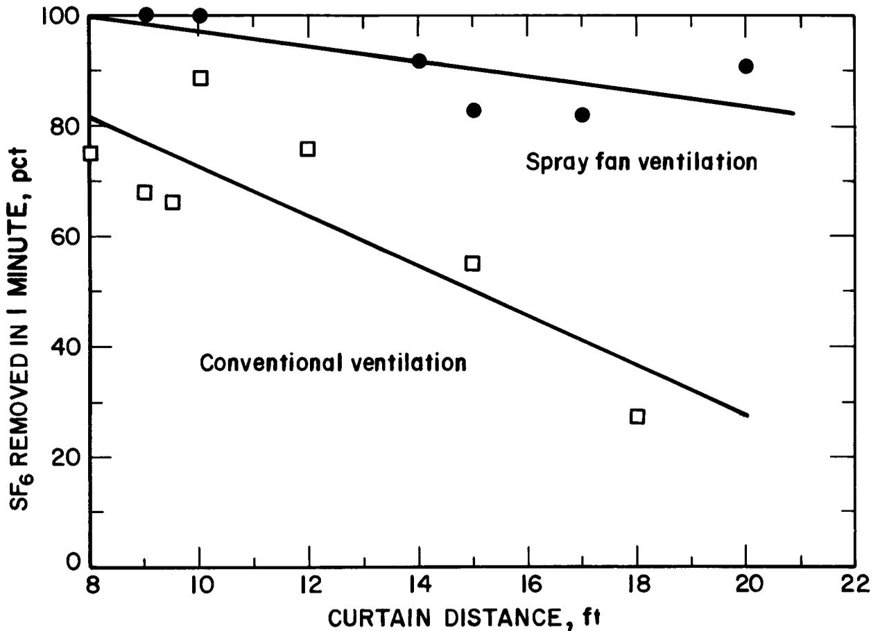
FIGURE 11. - Percent  $SF_6$  removed in 1 min versus curtain distance.
