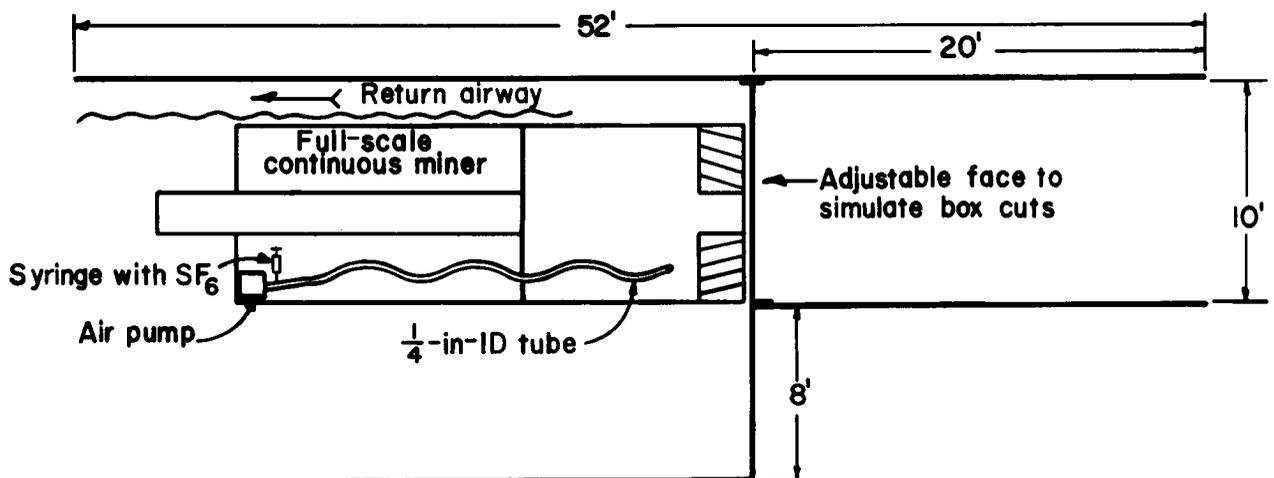
FIGURE 3. - Laboratory test setup for SF<sub>6</sub> studies.
