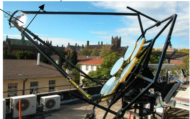
Figure 2: The high flux solar concentrator at the University of Sydney (6 mirror mode). The arrows indicate the x and y displacement as seen in Figure 1.
