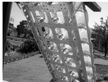
Figure 2. CPV for “Breeding Plants” that collects direct beam and provides diffused sunlight to the underneath plant.
