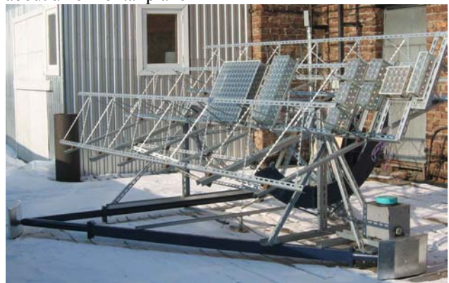
Figure 2: Sun tracker with concentrator PV modules installed on the roof of the Ioffe Institute. A similar tracker has been delivered to NREL (USA) and deployed in the frame of the IPP Program under Subcontract AAT-3-32614-01.
