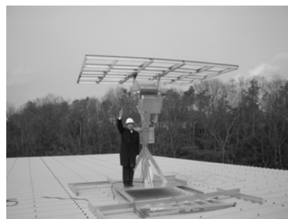
Figure 1. A new 3kW tracker developed by Daido Metal
