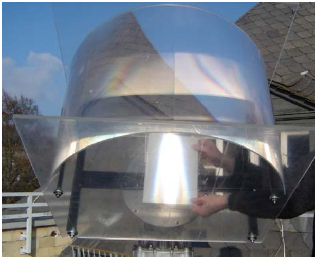
Figure 3: Nonimaging arched Fresnel. The reflective paper is held approximately at the receiver level, while the hands demonstrate the size of the concentrator
