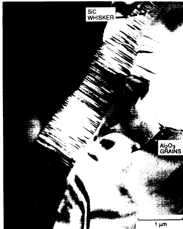
(a) Interface between whiskers and matrix is free from inclusions, large scale asperities, voids, etc. Alumina matrix grains visible.
