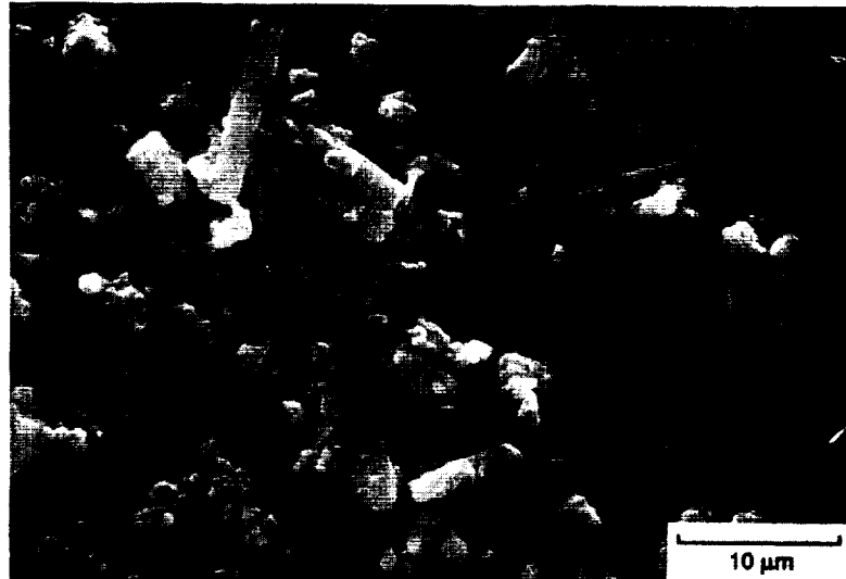
Figure 12. - Pulled-out whiskers from 1200 °C test. Note uniform whisker diameters and lack of seams distinguish these whiskers from debris "rolls".
