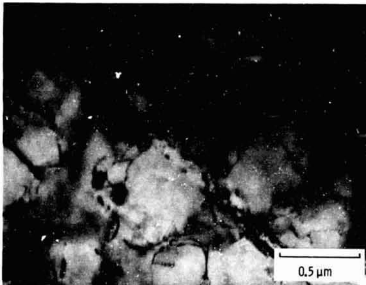
(c) \langle 111 \rangle reflection. (The small dark particles are carbides.)
