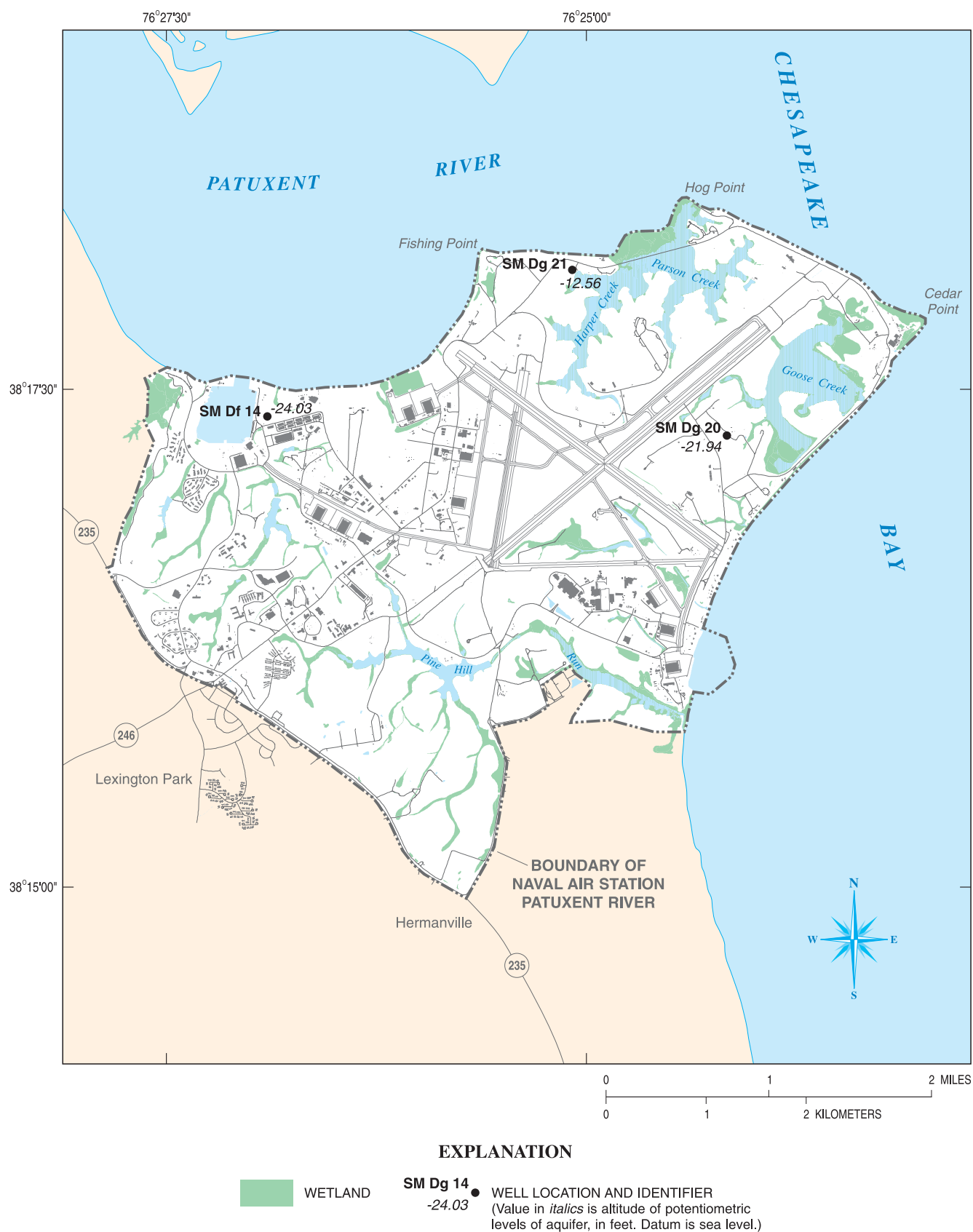
Figure 10. Altitude of the potentiometric levels of the Piney Point-Nanjemoy aquifer on April 20, 2000, Naval Air Station Patuxent River, Maryland.
