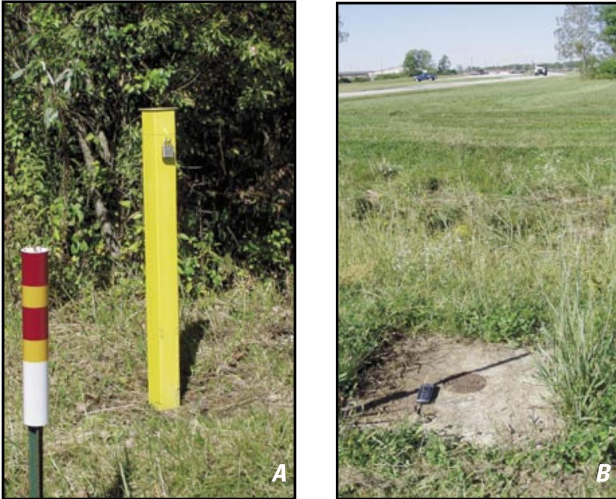
**Figure 7.** Photographs of (A) a piezometer with a protective cover and tubular marker and (B) a monitoring well with a flush-mount well vault at the U.S. Army Atterbury Joint Maneuver Training Center near Edinburgh, Indiana.
