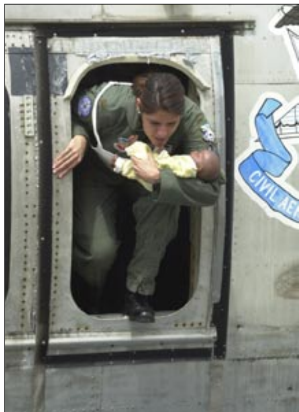
Figure 5. Infant carrier holds 2-month dummy horizontally as she climbs through the exit.
