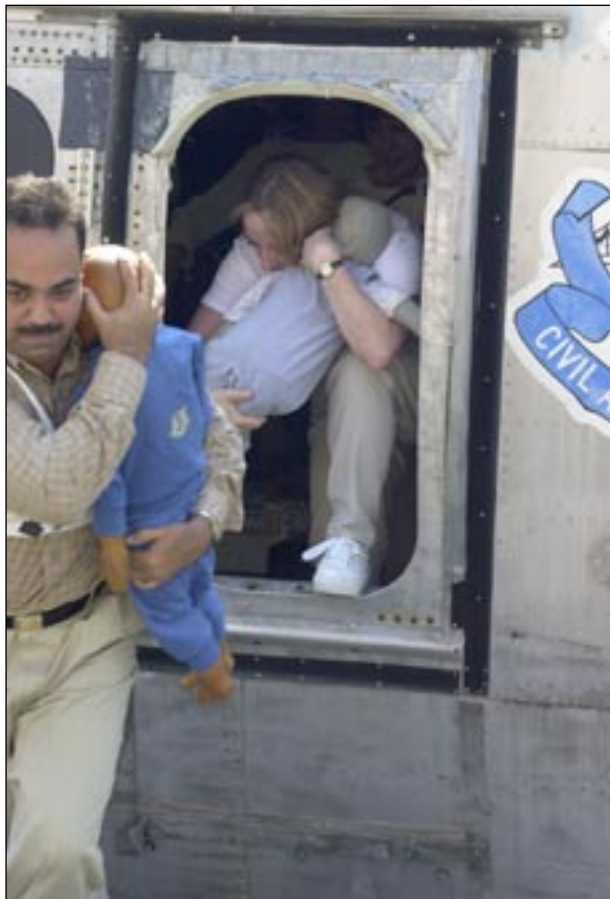
Figure 6. The head and neck of two 18-month dummies are well supported by infant carriers as they hold the infants vertically while evacuating.
