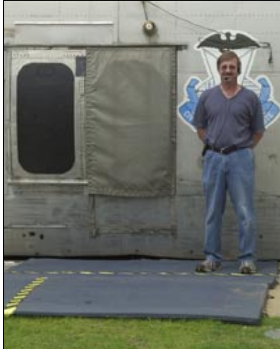
Figure 1. Test area shows Type III overwing exits and padded egress route. A canvas “hatch” was opened by a research team member.
