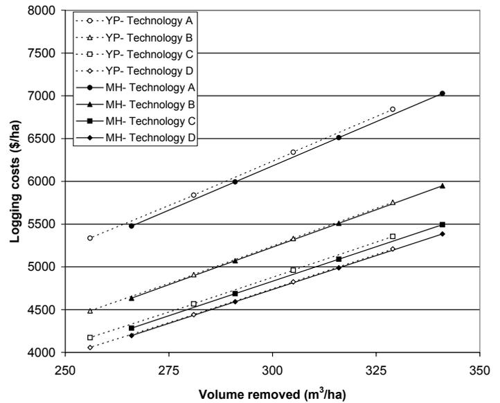
Figure 3.—Logging costs by volume removed for mixed hardwood and yellow-poplar stands for four different logging systems (see Table 3 and Page 3 for description of technologies used).
