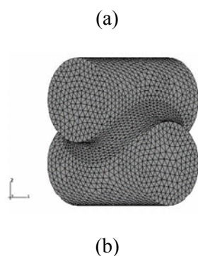
Figure 60. 3D modeling with fillet. Detail of the joint of a finite element model of two intersecting fibers with (a) d.o.i.=0.571 and (b) d.o.i.=0.667.
