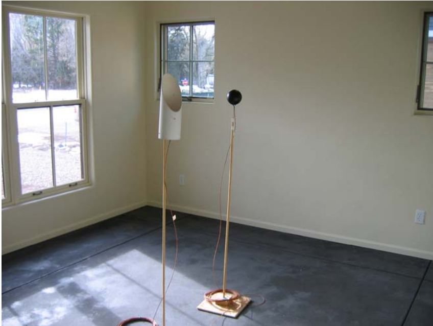
Figure 3. Shielded air temperature sensor (left) and black globe temperature sensor (right) in master bedroom.
