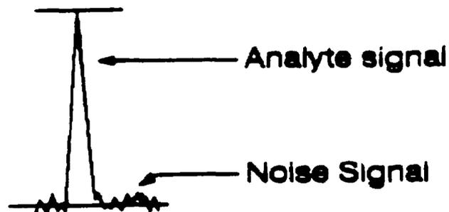
$$S/N = \frac{\text{Analyte Signal Peak Area}}{\text{Noise Signal Peak Area}}$$
