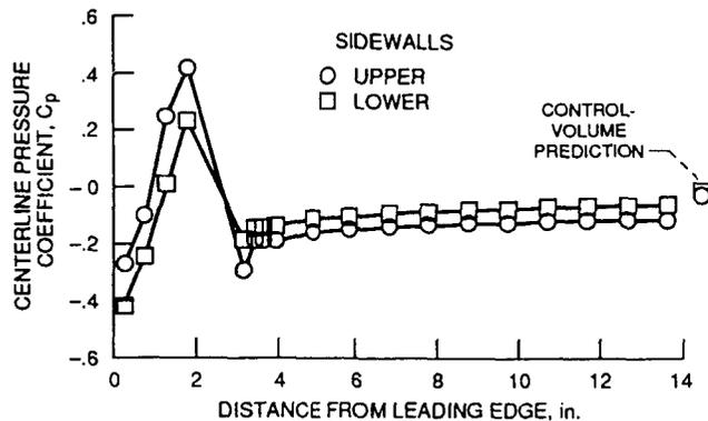
Fig. 23. Effect of sidewalls on ramp pressure distribution. Fuel pressure,  $P_f = 250$  psia; estimated jet penetration,  $Y_p, 0.30$ ; estimated equivalence ratio,  $\phi, 0.70$ .
