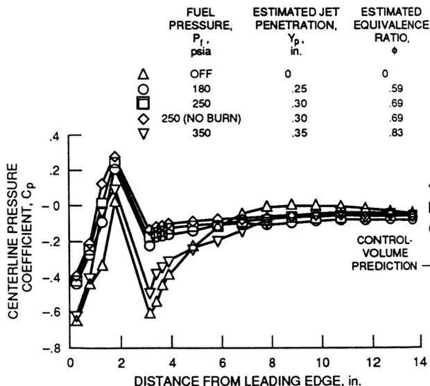
Fig. 19. Effect of increasing fuel pressure on ramp surface static pressure distributions. Free-stream static pressure,  $P_0$ , 8 psia.
