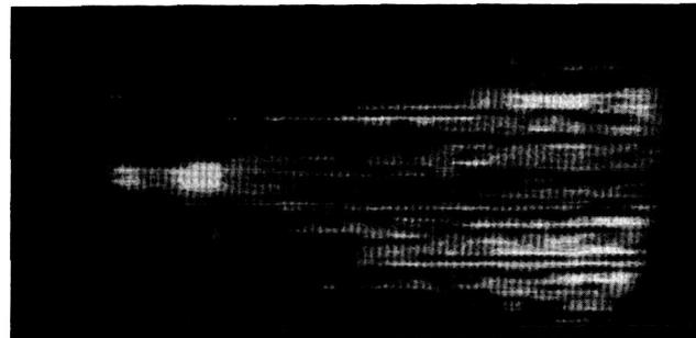
(b) Free-stream static pressure,  $P_0$ , 6 psia; free-stream total temperature,  $T_{t,0}$ , 540 °R; equivalence ratio,  $\phi$ , 0.51; jet penetration height,  $Y_p$ , 1.0 in.
