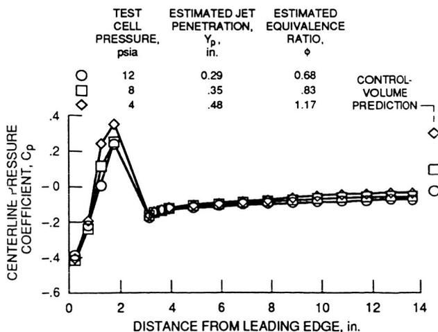
Fig. 20. Effect of increasing altitude on ramp surface static pressure distributions. Fuel pressure,  $P_f$ , 350 psia.
