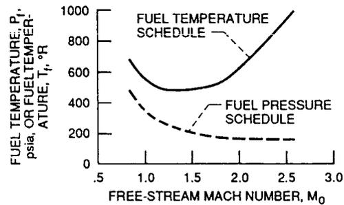
Fig. 7. Constant-equivalence-ratio ( $\phi = 1$ ) fuel injection schedule. Dynamic pressure at station 0,  $Q_0$ , 1000 lb/ft<sup>2</sup> abs; ratio of orifice spacing to orifice diameter,  $S/d^*$ , 7.56; ratio of orifice diameter to projected base height,  $d^*/Y_b$ , 0.00694.
