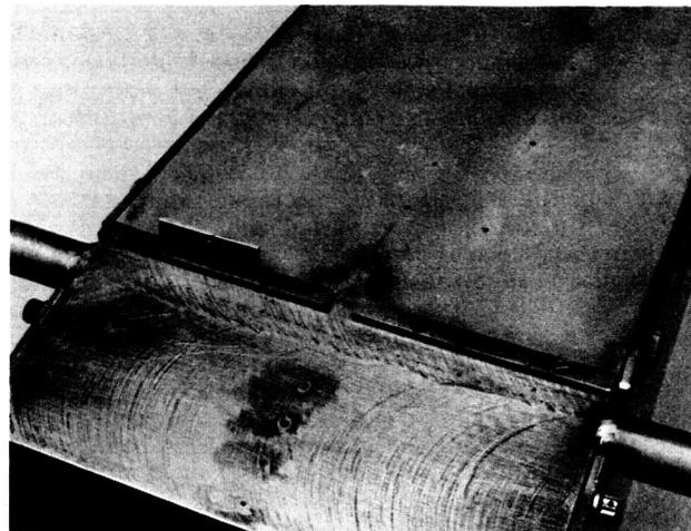
Fig. 17. Expansion ramp fuel injection and flameholding region.
