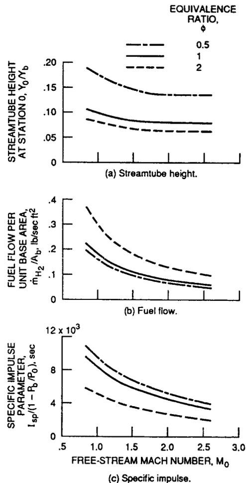
Fig. 6. Results for free-stream-pressure control volume. Dynamic pressure at station 0,  $Q_0$ , 1000 lb/ft<sup>2</sup> abs.
