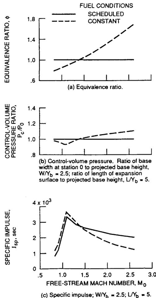
Fig. 8. Performance of example geometry. Dynamic pressure at station 0,  $Q_0$ , 1000 lb/ft<sup>2</sup> abs; ratio of orifice spacing to orifice diameter,  $S/d^*$ , 7.56; ratio of orifice diameter to projected base height,  $d^*/Y_b$ , 0.00694.
