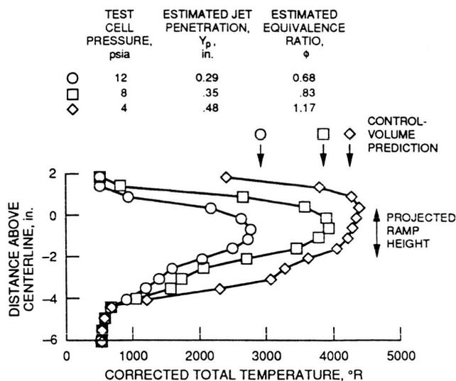
Fig. 21. Effect of increasing altitude on plume total temperature profiles. Fuel pressure,  $P_f$ , 350 psia.
