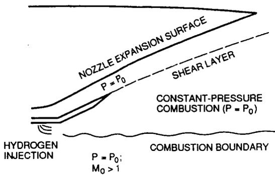
Fig. 4. Use of external burning with flap deflection to eliminate nozzle drag.
