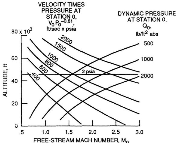
Fig. 14. Variation of DeZubay parameter with flight condition.
