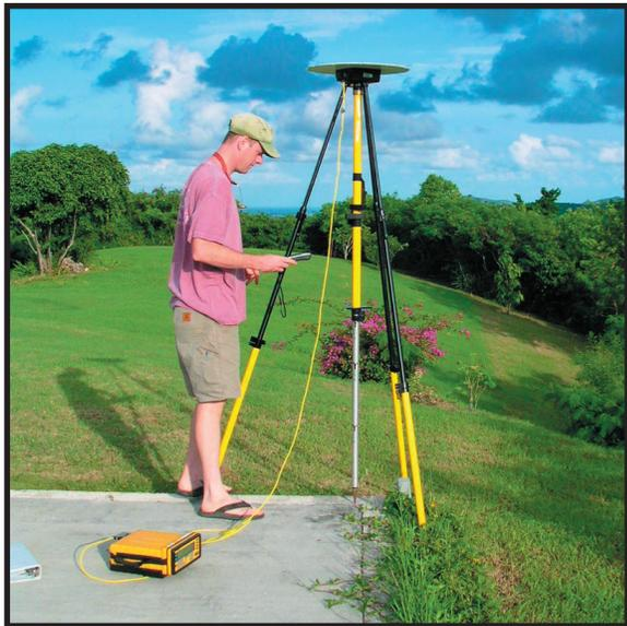
**Figure 2.2.** Taking GPS data to orthorectify aerial photographs.
