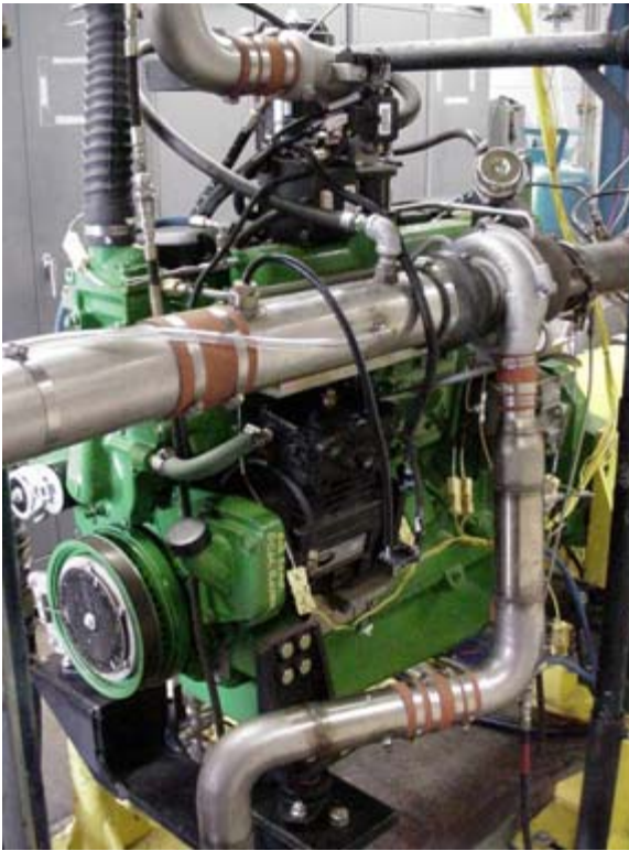
Photos 3-1 and 3-2. John Deere 8.1L deterioration factor engine installed on laboratory dynamometer at SwRI
