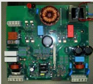
Hardware of PV-Inverter
