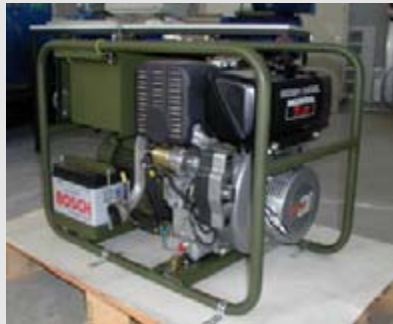
Single phase genset with ASG and capacitor (Fa. Kirsch)
