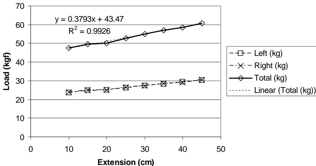
**Figure 5. Bungee load versus extension calibration curve. The lower curves represent the load and extension measured on each side. The upper curve is the sum of these two curves, representing the overall bungee system load versus extension curve.**
