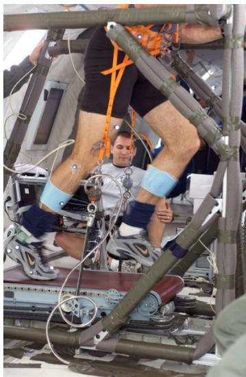
**Figure 3. Close-up of connection between harness and loading bungee illustrating load cell orientation during data collection.**
