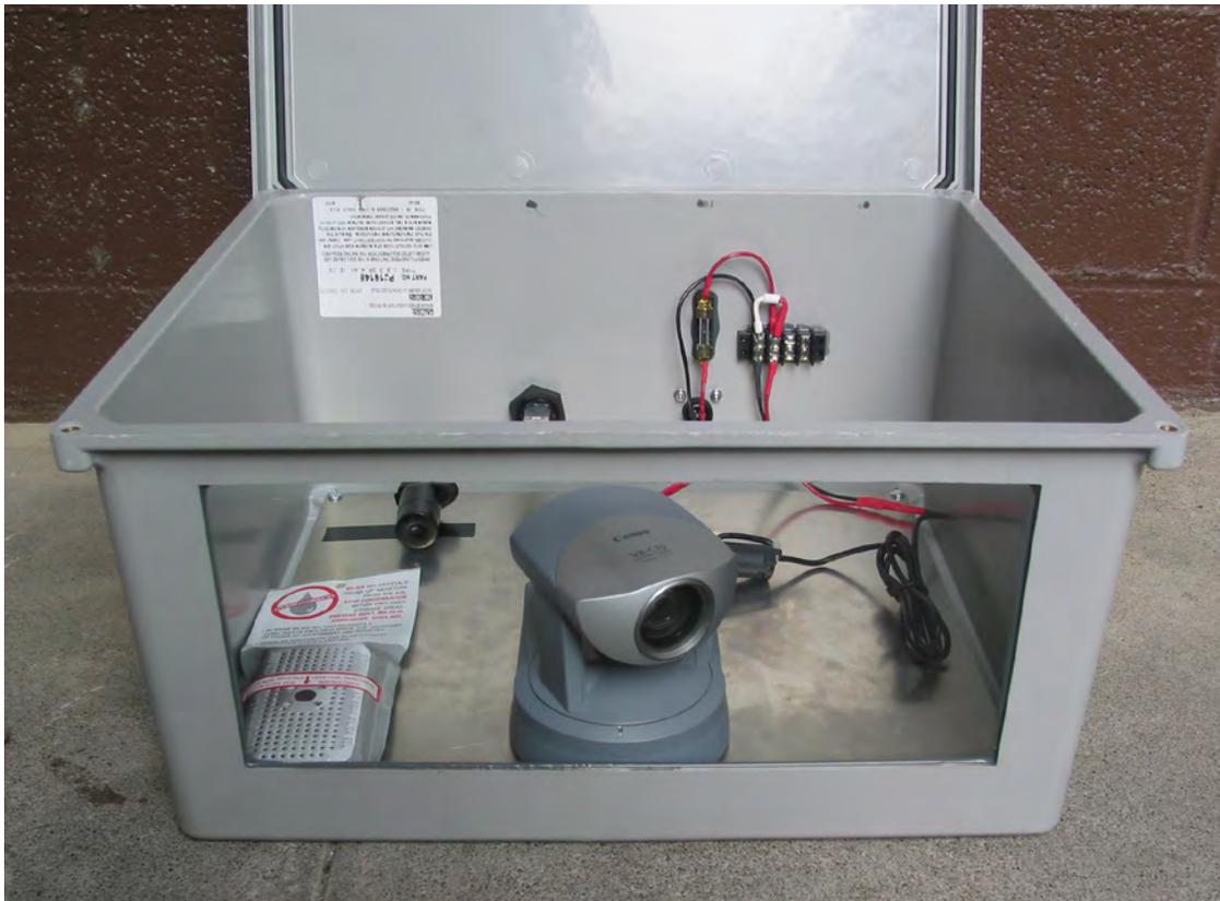
Figure 5. Canon VB-C10 network camera mounted inside a Hammond PJ16148H enclosure.
