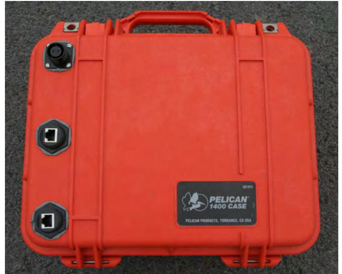
**Figure 11.** Cover of the Pelican APP-1400 enclosure containing the WRAP SBC and radio. The connector at the top of the photo is for power; the two lower connectors are RJ-45 bulkhead couplers.
