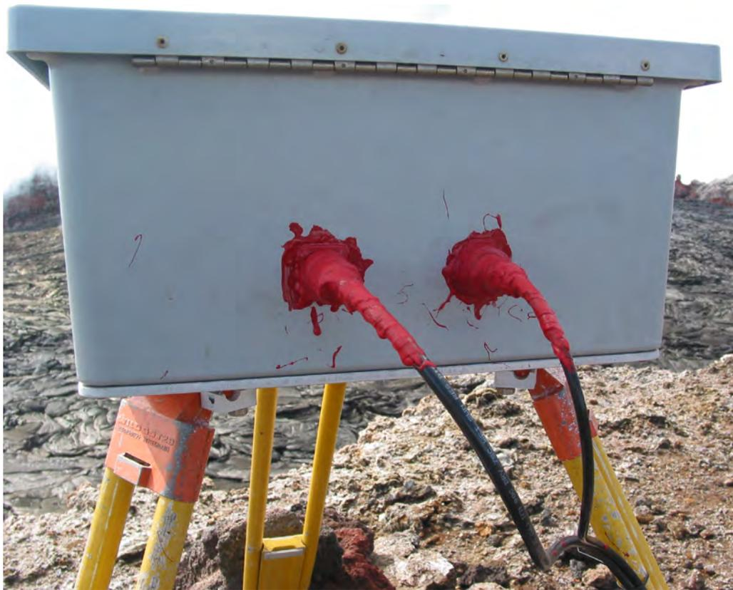
**Figure 6.** Camera enclosure and mounting tripod on the rim of Pu'u 'Ō'ō crater. The power and Ethernet connectors have been waterproofed with liquid electrical tape.
