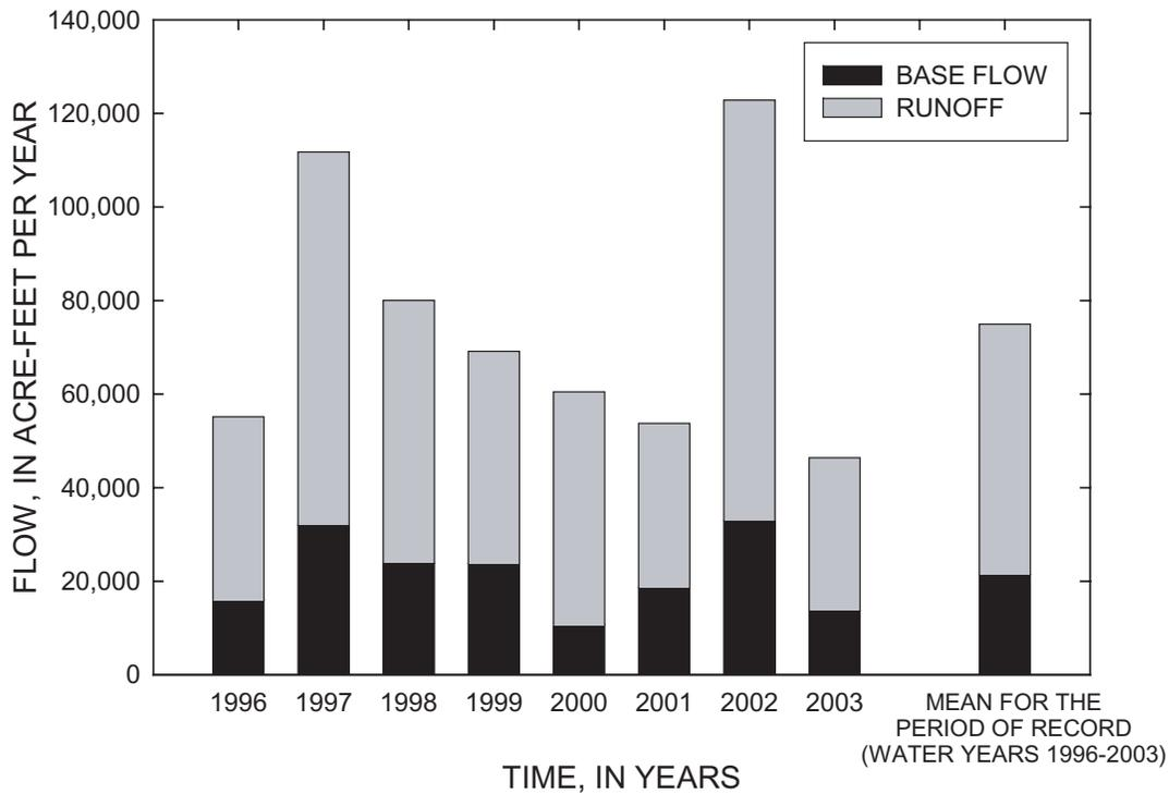
Figure 4. Base flow and runoff as components of total flow for 07055875 Richland Creek near Witts Springs, Arkansas.
