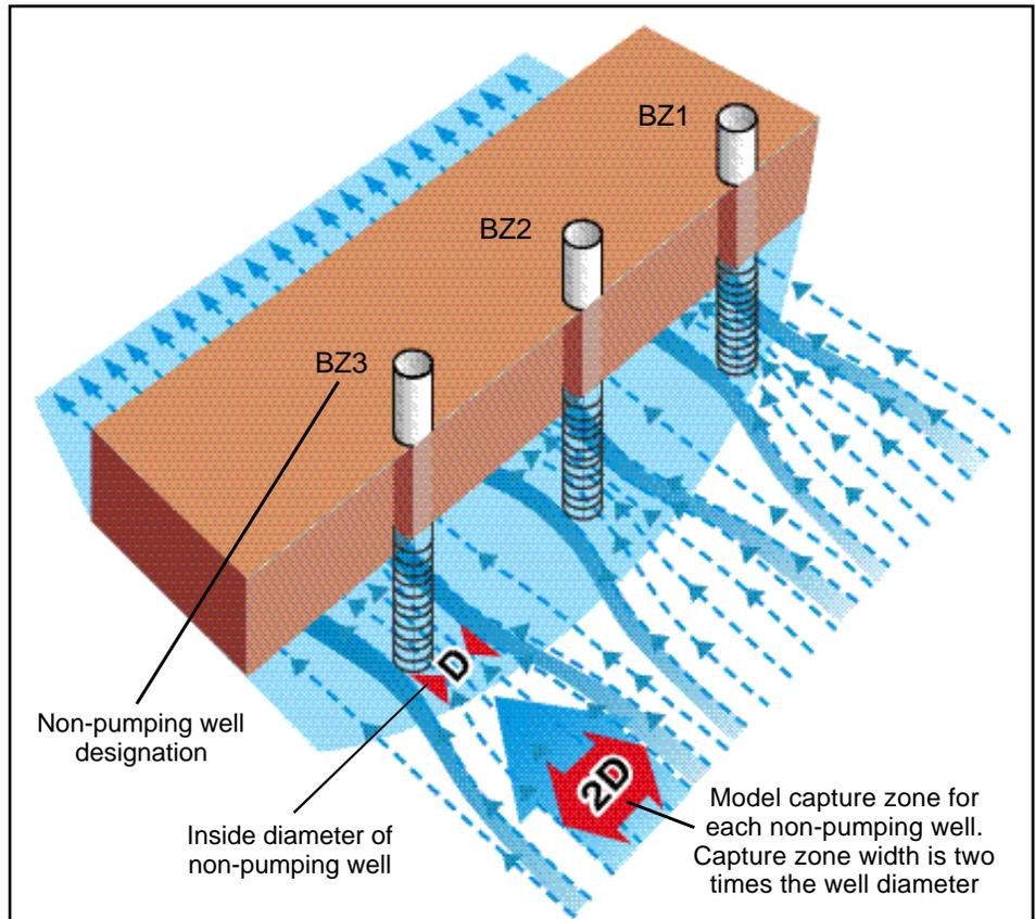
**Figure 1:** Schematic diagram showing non-pumping wells containing DARTs and modeled contaminant capture zones, Fry Canyon, Utah.
