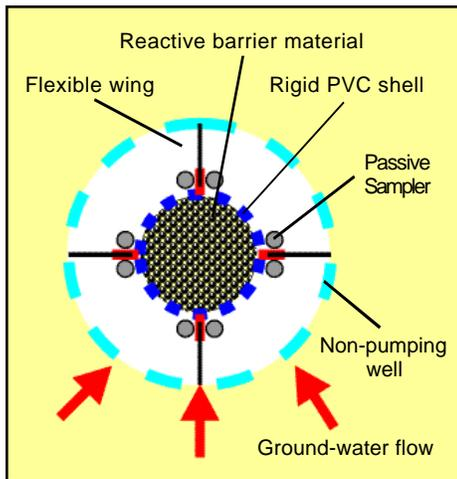
**Figure 2:** Schematic diagram of Deep Aquifer Remediation Tool (DART).
