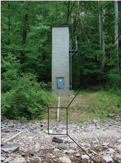
USGS streamgaging station at Big Bear Creek near Richfield (site 90, table 4), showing outside staff plate in dry streambed, June 19, 2002.
