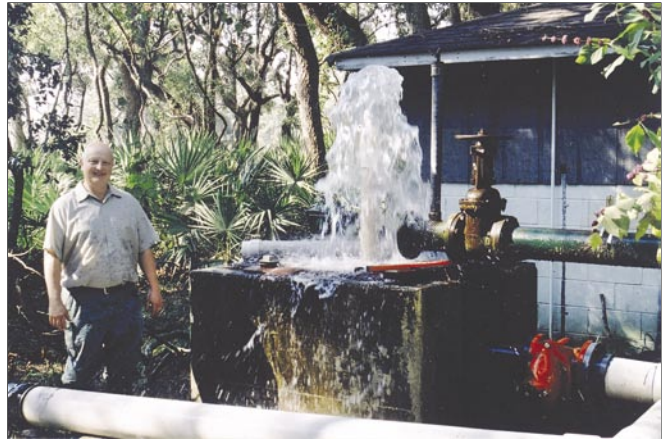
An unused production well on Jekyll Island is being converted into an observation well for continuous monitoring of ground-water levels. The 751-foot-deep well is completed in the Upper Floridan aquifer. Geophysical logs were collected to assess the integrity of the well casing and suitability for incorporation into the Georgia statewide ground-water-level monitoring network. A continuous ground-water-level recorder was installed at the well on October 25, 2004, at which time the water level was 21.83 feet above land surface. Photo by Michael F. Peck, USGS.
