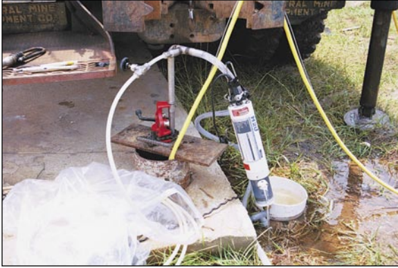
Water-quality sampling —Samples were collected from three wells to determine water quality. A pump is set into the well to collect the samples. Water-quality properties are monitored during the process of purging the well prior to sampling. Photo by Lester J. Williams, USGS.
