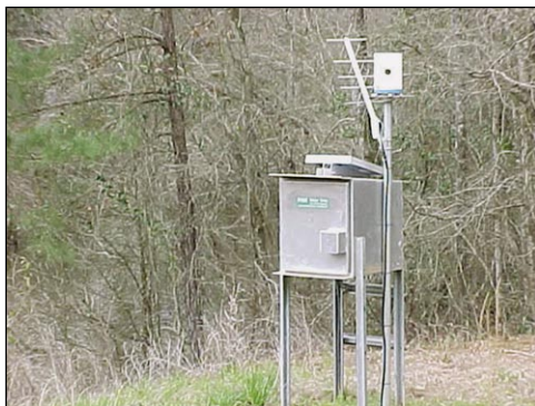
Real-time streamflow data-collection platform installed at station 02353265, Ichawaynochaway Creek at Georgia Highway 37, near Morgan, Georgia, and graph of data that can be accessed at http://ga.waterdata.usgs.gov/nwis/current/?type=flow&group_key=basin_cd
