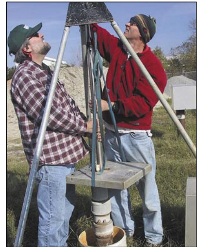
Geophysical logging and water-quality sampling of the Lower Floridan aquifer well 39Q024 on Tybee Island in Chatham County, December 2003. Photo by Edward H. Martin, USGS.
