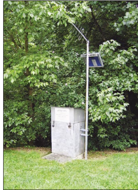
A typical real-time continuous recorder well in DeKalb County, which is part of the ground-water-level monitoring network. The equipment consists of a data logger, 30-pounds-per-square-inch transducer, a radio and antenna for transmitting data, and a solar panel and battery. Real-time data are typically recorded at 60-minute intervals, stored on site, and then transmitted to USGS offices from every 1 to 4 hours via satellite, telephone, or radio relay. The NWIS database may be accessed on the Web at http://waterdata.usgs.gov/ga/nwis/current/?type=gw Photo by Alan M. Cressler, USGS.
