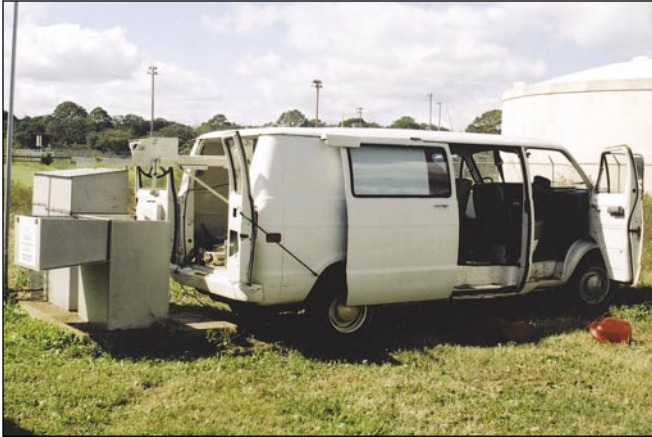
Fluid resistivity log being collected from an observation well completed in the surficial aquifer at Brunswick, Georgia. The log is being collected to determine the integrity of the well casing and to locate zones where saltwater may be entering the well. Photo by Michael F. Peck, USGS.
