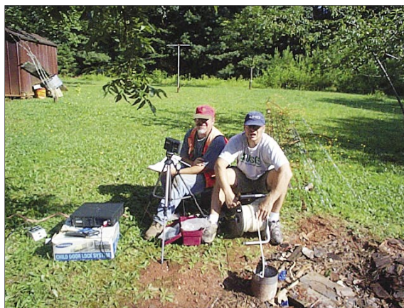
USGS personnel lower a video camera into well 14GG02 in the upper Apalachee River watershed. Photo by Phillip N. Albertson, USGS.
