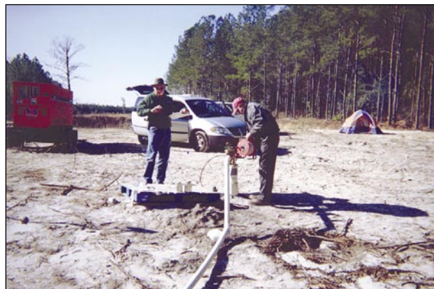
A USGS hydrologist and drilling contractor taking water-level measurements during aquifer test of the lower Brunswick aquifer at Old Sunbury Road, Liberty County, Georgia, January 2002. The test is being conducted to better define the hydraulic properties of the surficial and Brunswick aquifer systems and to determine the usefulness of these aquifers as secondary sources of ground water. Photo by Sherlyn Priest, USGS.
