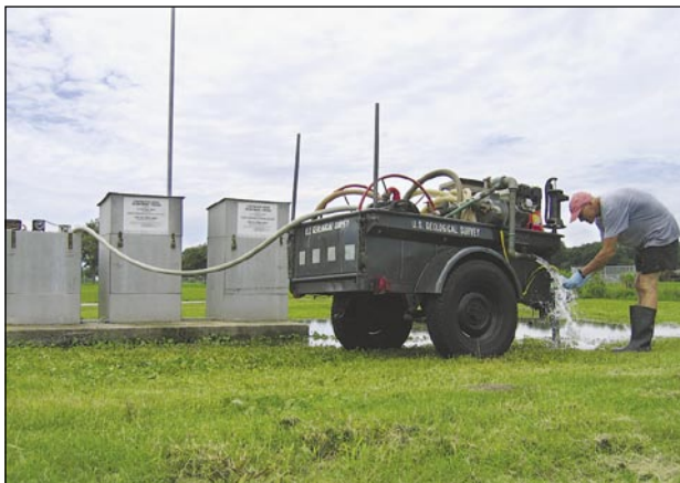
A hydrologic technician from the Ground-Water Information and Project Support Unit collects a water sample for chloride analysis from a well in Glynn County, Georgia. The sampling trailer contains a 5-horsepower centrifugal pump, reel with 100 feet of suction hose, and pipe fittings and adapters. The samples are collected annually in support of the Brunswick and Glynn County Cooperative Water-Resources Program. Photo by Alan M. Cressler, USGS.
