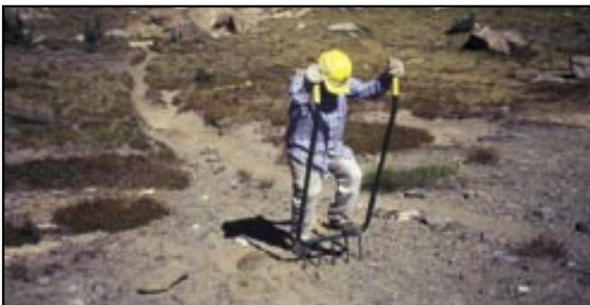
Figure 3–27—The U-bar digger is used to break up compacted soil.
