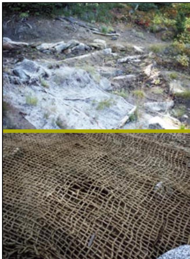
Figures 3–137a and 137b—Ten years of exposure to sun and weather in the subalpine zone of Washington has not decomposed this jute netting (top). Jute (bottom) is no longer used in such settings.
