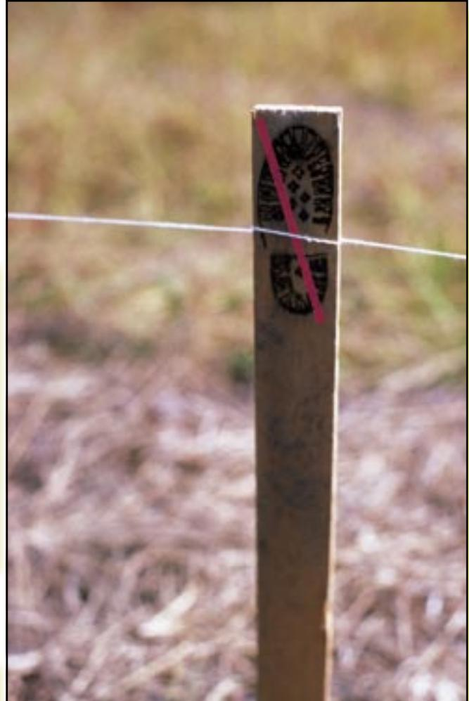
Figure 3–85c—Specially marked stakes are more durable.
