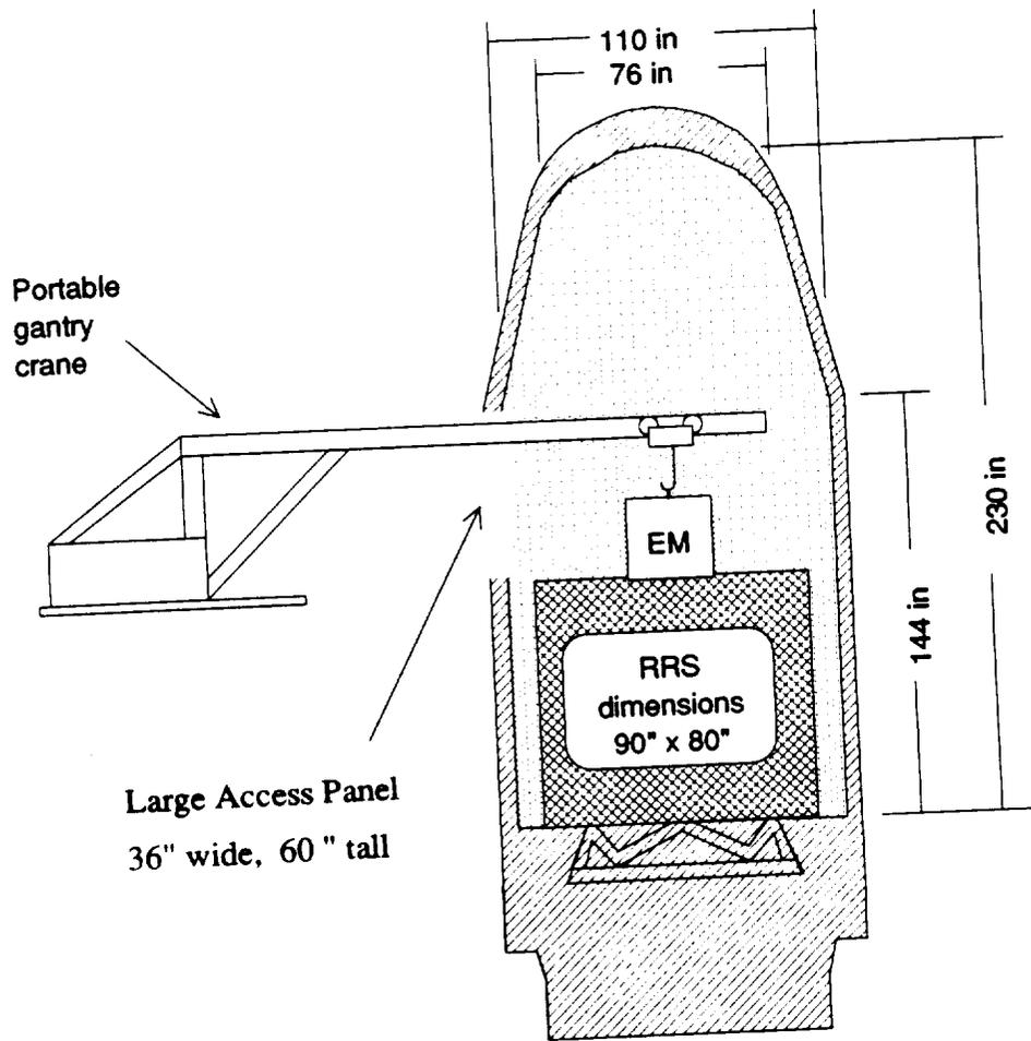
Figure 8-5. Delta Late EM Installation Scenario (ROSAT Fairing)
