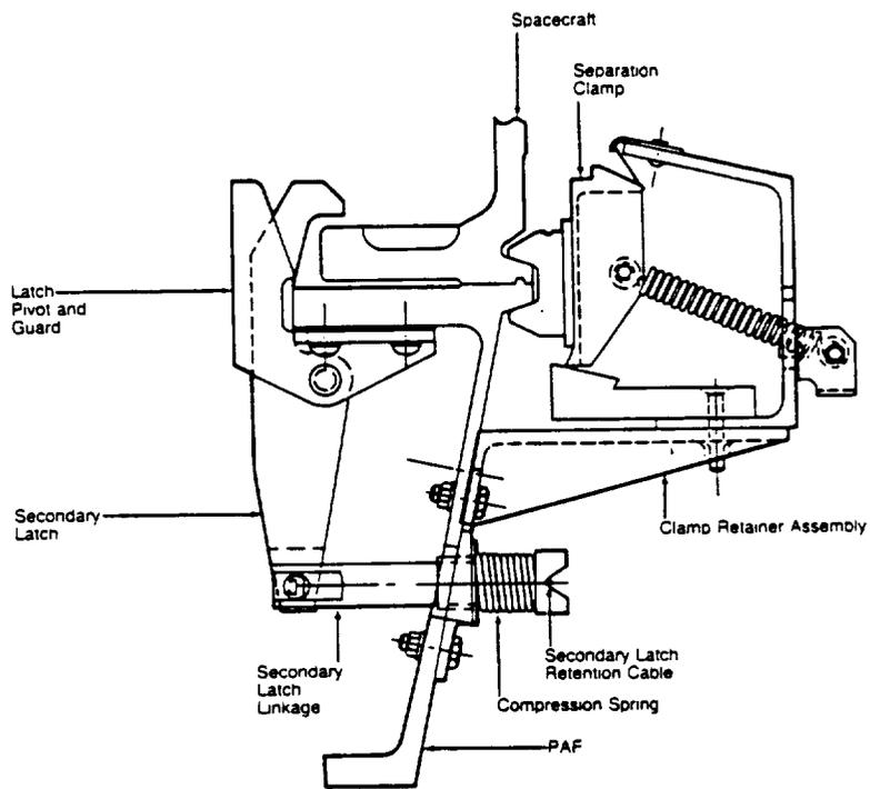
Figure 8-6. Delta PAF Clamp Release
