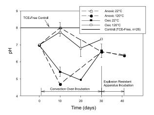
Figure 4.8 The pH of anoxic (Batch 4) and oxic (Batch 3) ampules with 100 mg/L of TCE and TCE-free controls stored at 22°C and incubated at 120°C.
