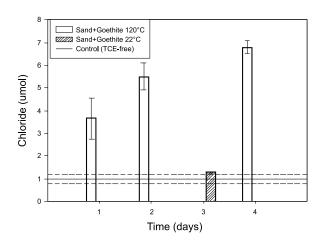
Figure 4.21 Amount of chloride in anoxic ampules with Ottawa sand+1% goethite and 100 mg/L TCE (Batch 7) stored at 22°C and incubated at 120°C.
