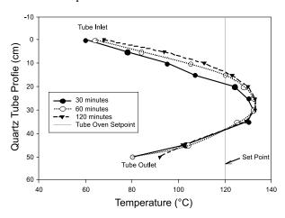
**Figure A.1** Temperature profile within the quartz tube heated to 120°C.
