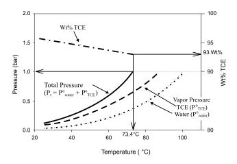
**Figure 2.1** Water and TCE-NAPL vapor pressure as a function of solution temperature at 1 bar or 1.02 atm of total gas phase pressure.
