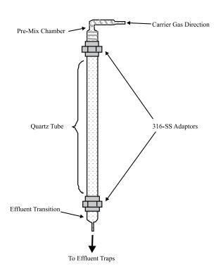
**Figure 3.1** Quartz tube experimental apparatus.
