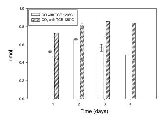
**Figure 4.16** Amounts of CO and  $CO_2$  in anoxic ampules amended with NaOH (0.26 mM) to pH 10 (Batch 5) and 100 mg/L of TCE incubated at  $120^{\circ}$ C.
