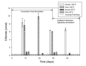
**Figure 4.19** Amount of chloride in anoxic (Batch 4) and oxic (Batch 3) ampules with 100 mg/L of TCE stored at 22°C and incubated at 120°C.
