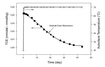
**Figure 2.5** Measured concentration of TCE vs. time for Experiment TCE-40 and radical chain reaction model fit.
