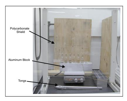
**Figure 4.2** Explosion-resistant ampule incubation apparatus.
