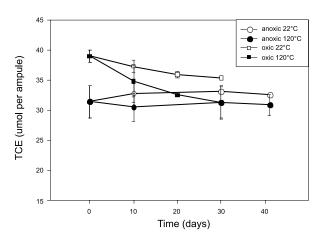
**Figure 4.4** Amount of TCE in the 100 mg/L anoxic (Batch 4) and oxic (Batch 3) ampules stored at 22°C and incubated at 120°C.
