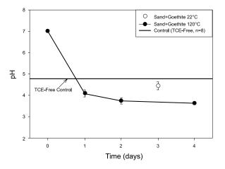
**Figure 4.10** The pH of anoxic ampules that contained acid-washed Ottawa sand+1% goethite with 100 mg/L of TCE (Batch 7) and TCE-free controls stored at 22°C and incubated at 120°C.
