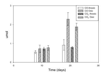
**Figure 4.12** Amounts of CO and  $CO_2$  in anoxic (Batch 1) and oxic (Batch 2) ampules with 1,000 mg/L of TCE and incubated at  $120^{\circ}$ C.
