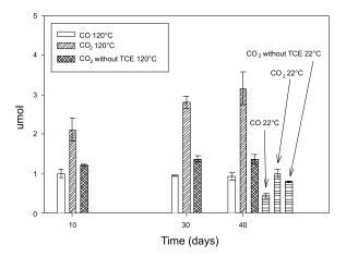
**Figure 4.14** Amounts of CO and CO<sub>2</sub> in anoxic ampules with Ottawa sand and 100 mg/L of TCE (Batch 6) stored at 22°C and incubated at 120°C.
