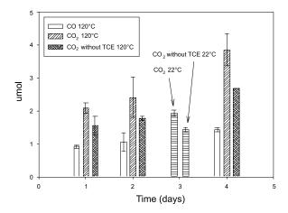
**Figure 4.15** Amounts of CO and CO<sub>2</sub> in anoxic ampules with Ottawa sand+1% goethite and 100 mg/L of TCE (Batch 7) stored at 22°C and incubated at 120°C.
