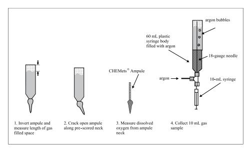
**Figure 4.3** Illustration of the ampule gas sample collection method.
