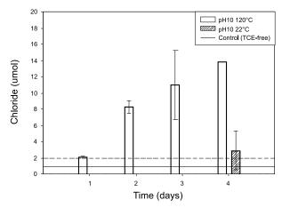
**Figure 4.22** Amount of chloride in anoxic ampules amended with NaOH (0.26 mM) to pH 10 with 100 mg/L of TCE (Batch 5) stored at 22°C and incubated at 120°C.
