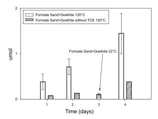
Figure 4.28 Amount of formate in anoxic ampules with Ottawa sand+1% goethite and 100 mg/L of TCE (Batch 7) stored at 22°C and incubated at 120°C.
