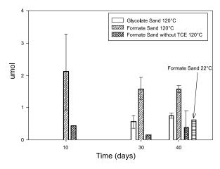
**Figure 4.27** Amount of glycolate and formate in anoxic ampules with Ottawa sand and 100 mg/L of TCE (Batch 6) stored at 22°C and incubated at 120°C.
