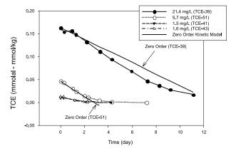
**Figure 2.2** Measured concentration of TCE vs. time along with the zero-order reaction model fit.
