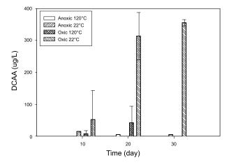
**Figure 4.23** Concentration of dichloroacetate (DCAA) in the anoxic (Batch 1) and oxic (Batch 2) ampules with 1,000 mg/L of TCE stored at 22°C and incubated at 120°C.
