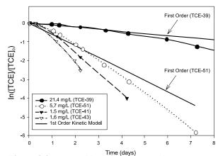
Figure 2.3 Natural log of the measured TCE concentration normalized by the initial TCE concentration vs. time along with the first-order reaction model fit.
