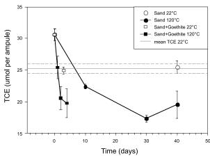
Figure 4.5 Amount of TCE in anoxic 100 mg/L ampules with Ottawa sand (Batch 6) and Ottawa sand+1% goethite (Batch 7) stored
