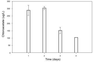
**Figure 4.24** Concentration of chloroacetate in ampules amended with NaOH (0.26 mM) to pH 10 and 100 mg/L TCE (Batch 5) incubated at 120°C.
