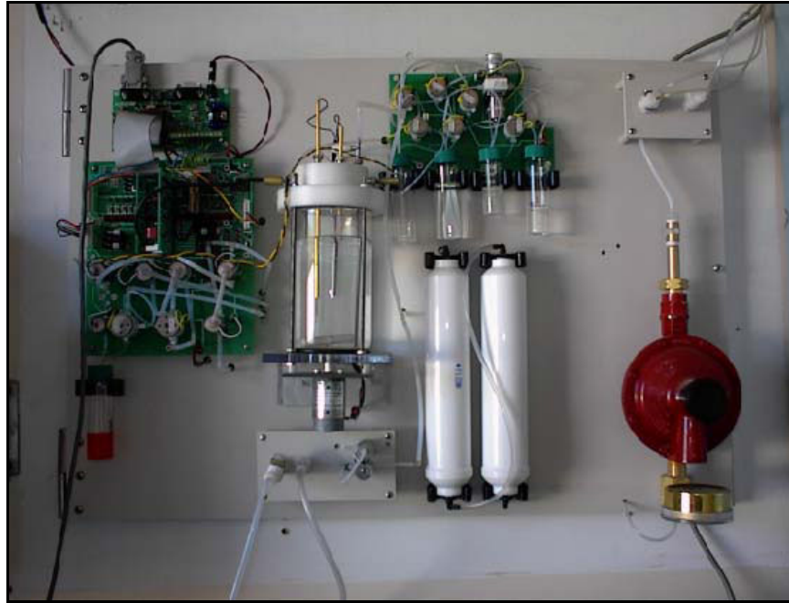
Indoor Wall-Mounted Sampling and Analysis System for Process Monitoring. Source: Burge Environmental
