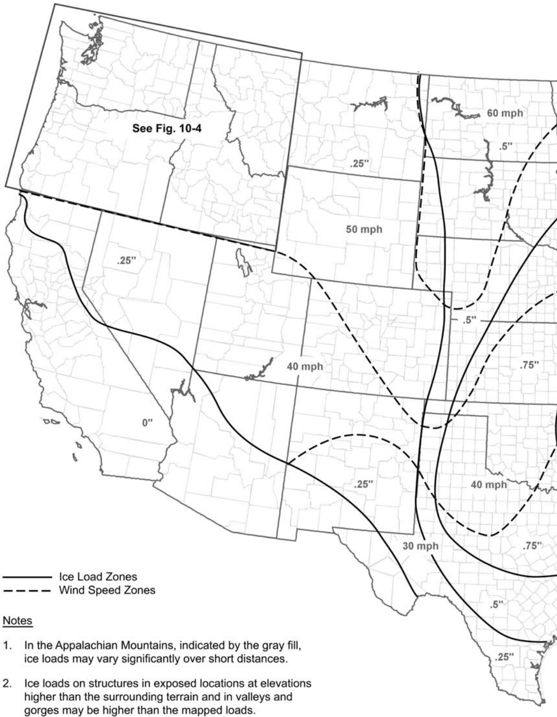
Figure 1. Uniform radial ice thicknesses due to freezing rain, with concurrent 3-s gust speeds, for a 50-year return period a) western United States
