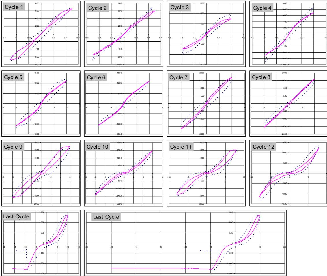
Figure 4-30 Cycle-By-Cycle  $Q_x - D_x$  Relation For Cross Loading
