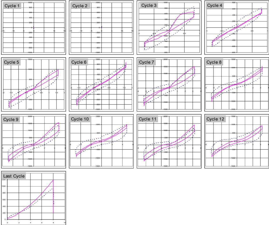
Figure 4-25 Cycle-By-Cycle  $Q_y - D_y$  Relation For Rectangular Loading
