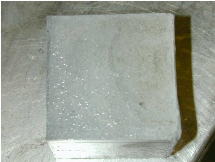
**Figure 5.8** Cube specimen after 1 month in  $\text{Na}_2\text{HPO}_4$ .
