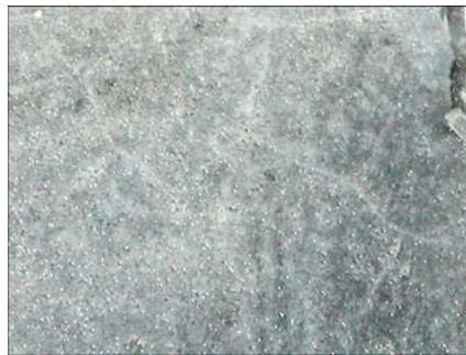
**Figure 5.43** Carbonate crystal deposits on surface of specimen cured in  $\text{Na}_2\text{HPO}_4$ .
