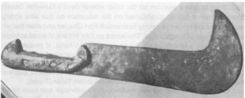
FASCINE KNIFE. Sappers and miners used knives of this type to cut twigs and branches for fascines.
