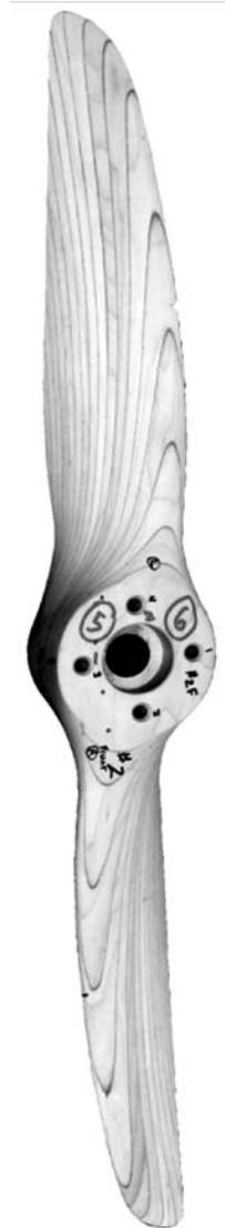
Figure 1—An unfinished wood propeller provided to the Forest Products Laboratory for evaluation.
