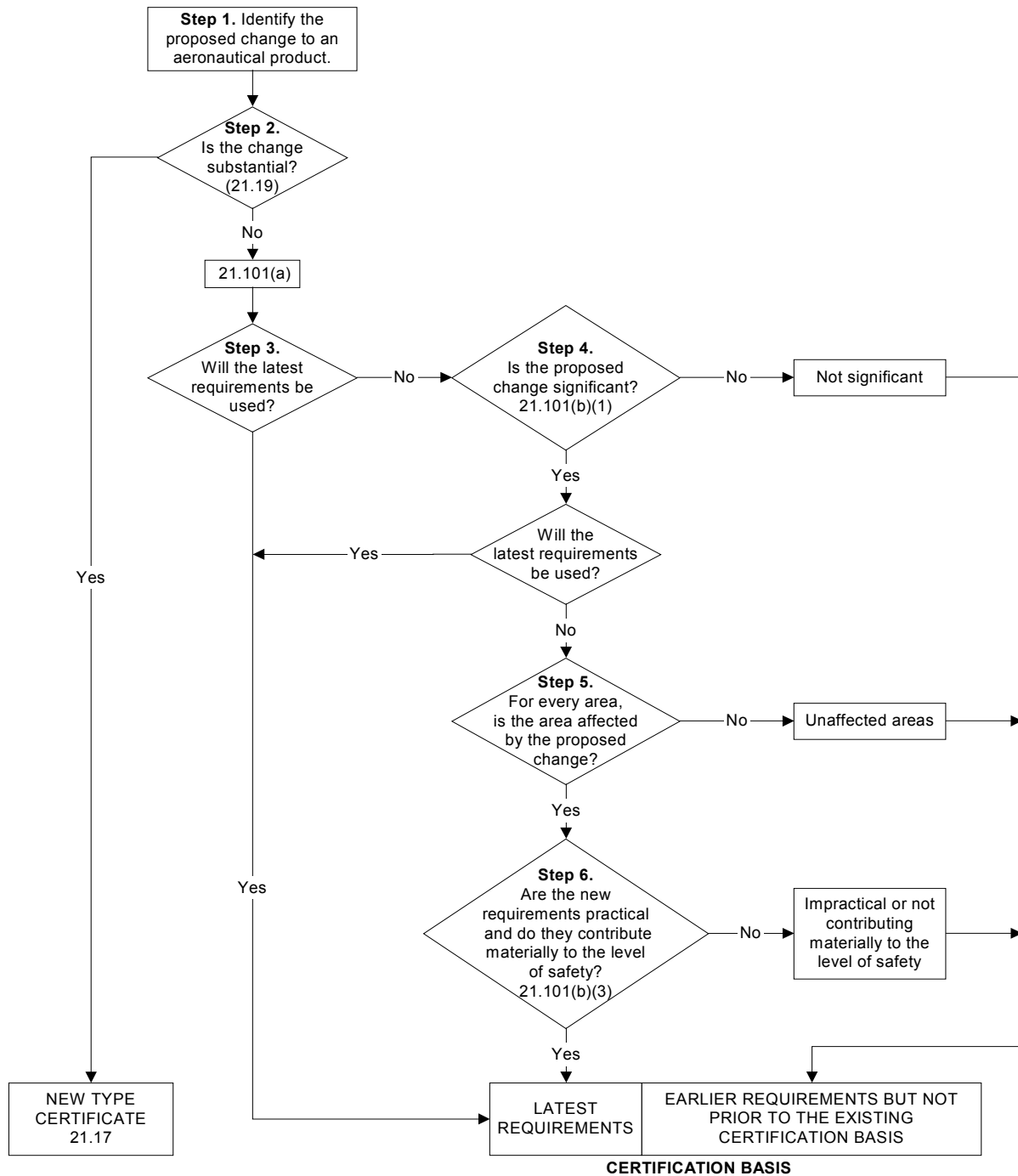
FIGURE 1: ESTABLISHING THE CERTIFICATION BASIS FOR CHANGED PRODUCT
