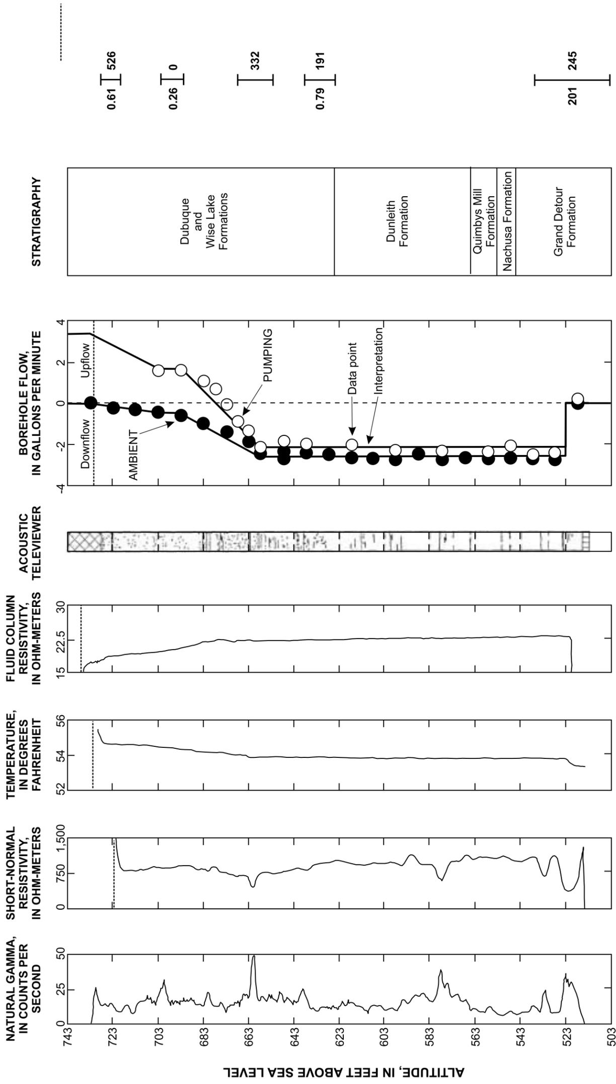
**Figure 6.** Natural-gamma, short-normal resistivity, fluid temperature, fluid-column resistivity, acoustic-televviewer, and flowmeter logs; stratigraphy; horizontal hydraulic conductivities; and total concentration of volatile organic compounds in the test intervals isolated with a packer assembly for borehole G134GP in the vicinity of the Parson's Casket Hardware Superfund site, Belvidere, Ill. (See figure 1 for location of borehole.)
