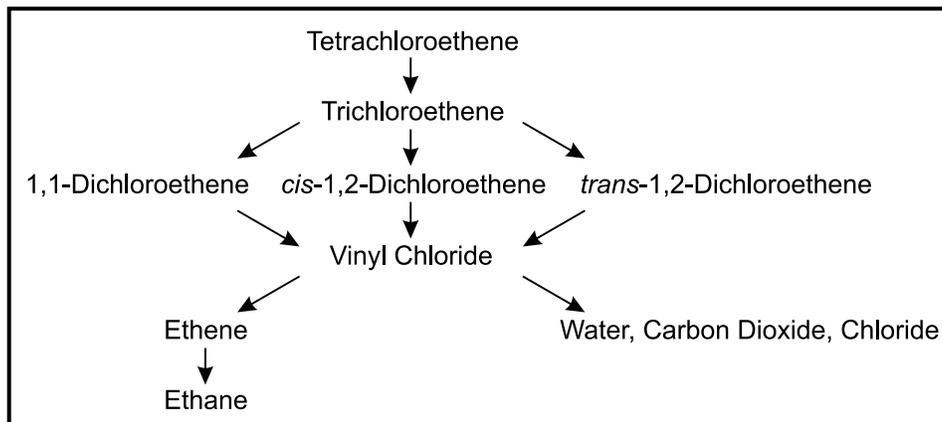
Figure 14. Reductive dechlorination sequence for chlorinated ethenes.
