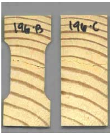
Figure 12—Example of dog-bone and wafer specimen failures. These specimens have growth ring angles of 22.5°.
